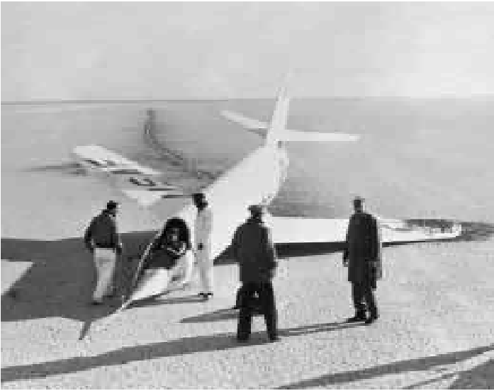
NASA Photo E-749. X-2 on lakebed after landing on skids.
