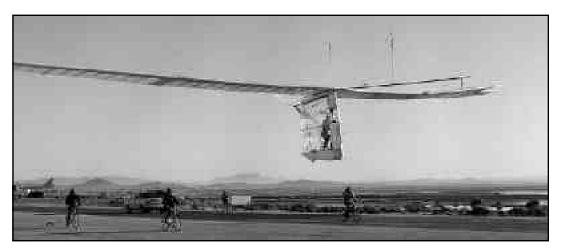
During the early part of 1980, in a joint project with NASA's Langley Research Center and AeroVironment, NASA's Dryden Flight Research Center gathered data on a Gossamer Albatross in which the lightweight aircraft flew under three conditions: using human power, using a small electric motor, and in a towed condition with the propeller removed. NASA photo ECN 12558
