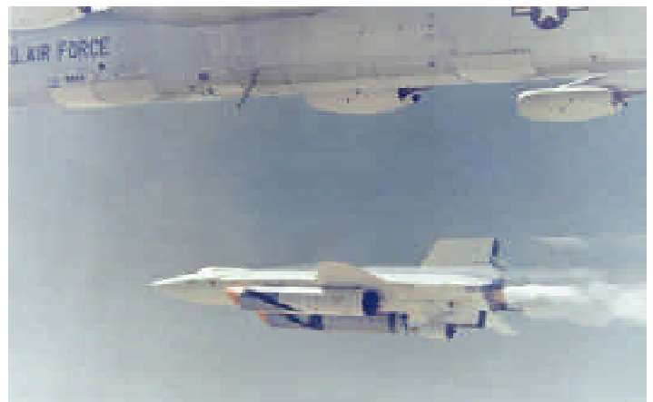
X-15A-2 (with ablative coating and external tanks) in which Pete Knight set the unofficial world speed record. NASA photo EC68 1899
