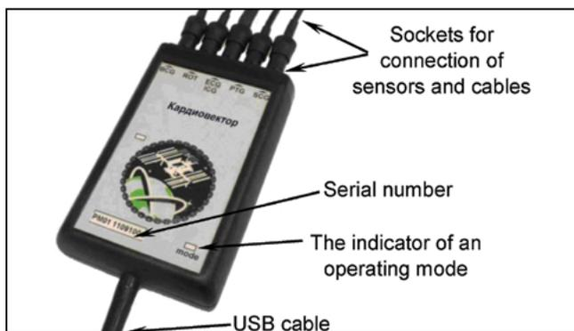
Figure 9. Cardiovector device worn by cosmonauts on ISS to measure cardiac activity. Image adapted from Baevsky, *Acta Astronautica*.
