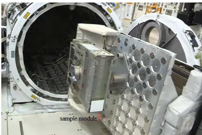
Figure 19. ExHAM sample module irradiated with trapped high-energy electrons. Image adapted from Bel, *Journal of Applied Polymer Science*.
