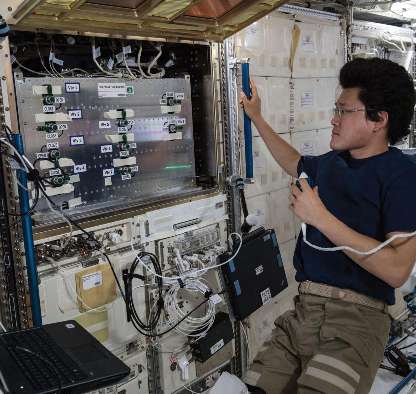
*JAXA crew member Norishige Kanai in the Japanese Experiment Module aboard the ISS while working with the Two-Phase Flow experiment. Two-Phase Flow examines the behavior of bubbles, liquid-vapor flow, and heat transfer in microgravity. iss055e098144.*
