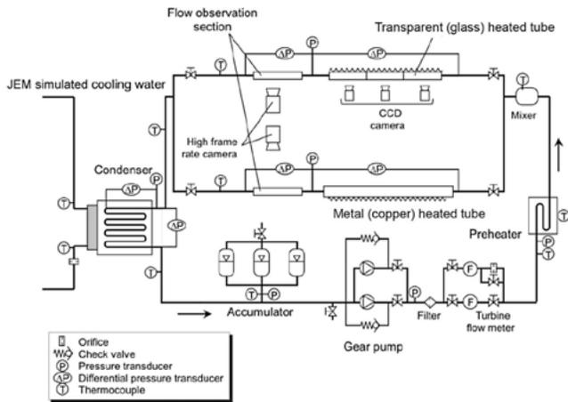
Figure 17. Diagram of test loop of Two-Phase Flow. Image adapted from Inoue, *Microgravity Science and Technology*.
