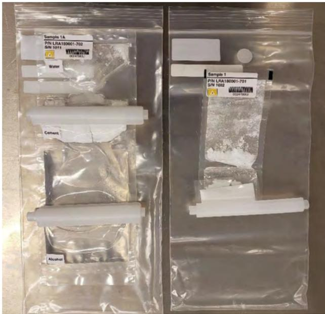
Figure 20. On the left, a pouch containing the cement and gypsum mix along with alcohol to stop the hydration reaction when needed. On the right, a pouch containing the cement and gypsum mix left to hydrate for the duration of the flight. Image adapted from Collins, *Construction and Building Materials*.
