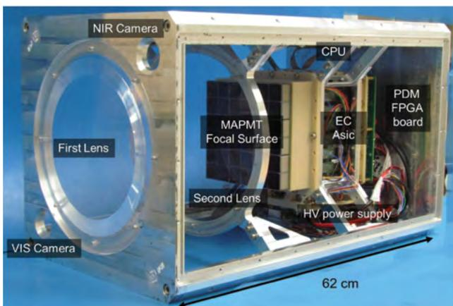
Figure 14. Mini-EUSO mock-up displaying three main compartments (optics, focal surface, and data acquisition). Image adapted from Bacholle, *The Astrophysical Journal Supplement Series*.
