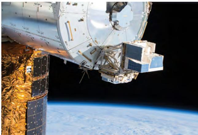
Figure 22. View of ASIM attached externally to the ISS. NASA image iss057e055409.
