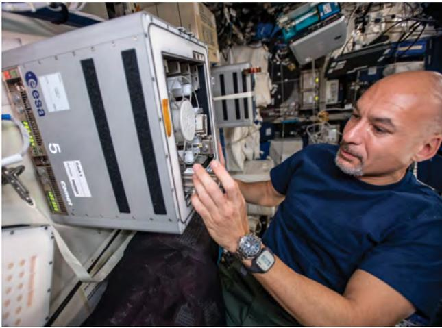
Figure 7. ESA astronaut Luca Parmitano at the BioRock Experimental Unit aboard the ISS. An experiment container is being inserted into the KUBIK incubator for sample processing. Image adapted from Cockell, *Nature Communications*.
