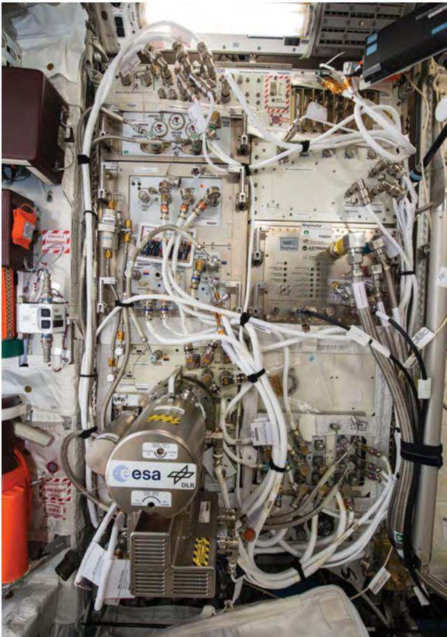
Figure 15. Electromagnetic Levitator in the Columbus module of ISS. NASA image: iss041e096097.
