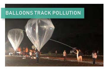
NASA and the Indian Space Research Organization (ISRO) sponsor a study of the Asian Tropopause Aerosol Layer (ATAL), an area of enhanced aerosol particles that appears in the summertime. Using balloon-lofted instruments, the "Balloon measurement campaign of the Asian Tropopause Aerosol Layer (BATAL)" collects data to better understand this seasonal atmospheric phenomenon and its potential impact on water resources, ozone, weather and climate.
