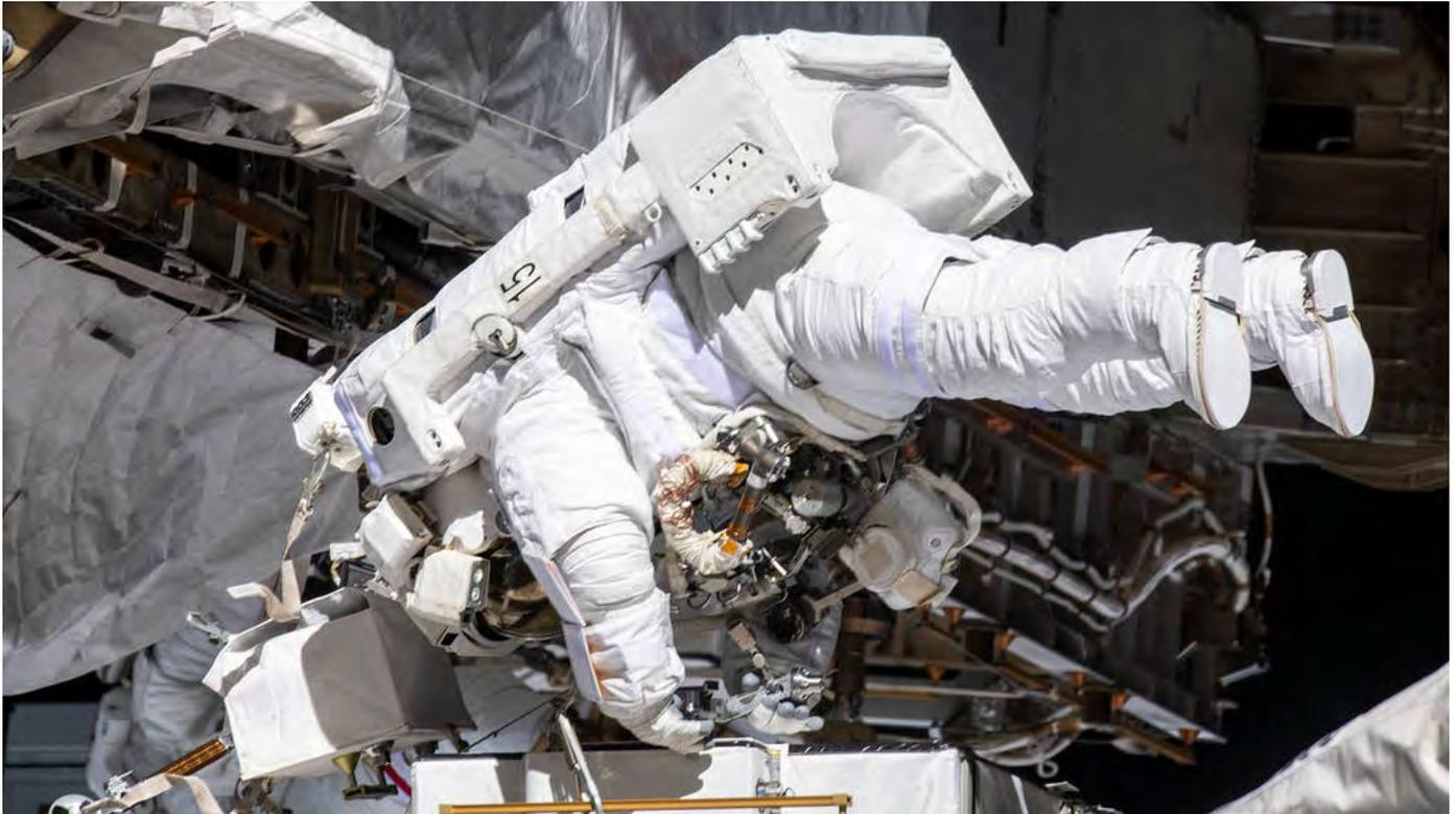
Astronaut Christina Loch works in the vacuum of space while tethered near the Port 6 truss segment of the International Space Station to replace older hydrogen-nickel batteries with newer, more powerful lithium-ion batteries, during the October 11, 2019, spacewalk. Fellow NASA astronaut Andrew Morgan (out of frame) assisted Koch during the six-hour and 45-minute spacewalk. **Photo Credit: NASA**
