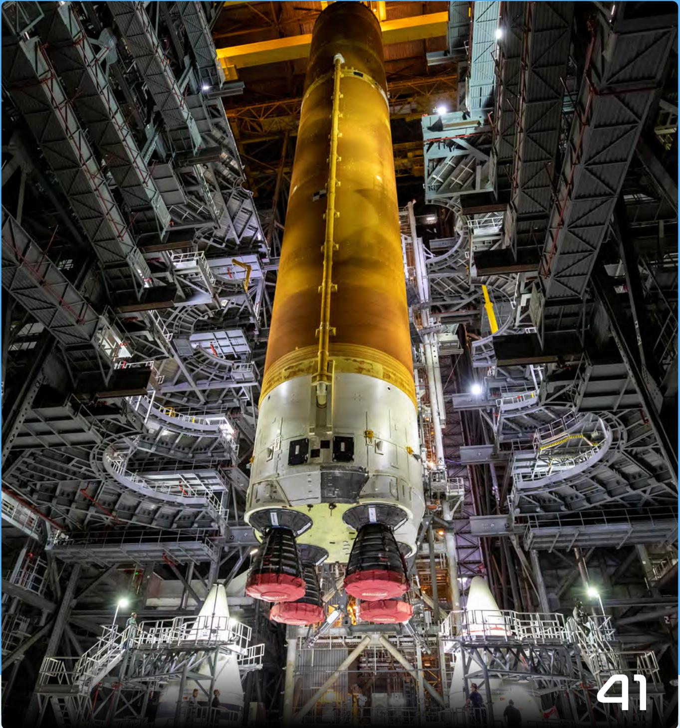
Teams with NASA's Exploration Ground Systems and contractor Jacobs prepare to lower the Space Launch System (SLS) core stage – the largest part of the rocket – onto the mobile launcher, in between the twin solid rocket boosters, inside High Bay 3 of the Vehicle Assembly Building at NASA's Kennedy Space Center in Florida on June 12, 2021.
