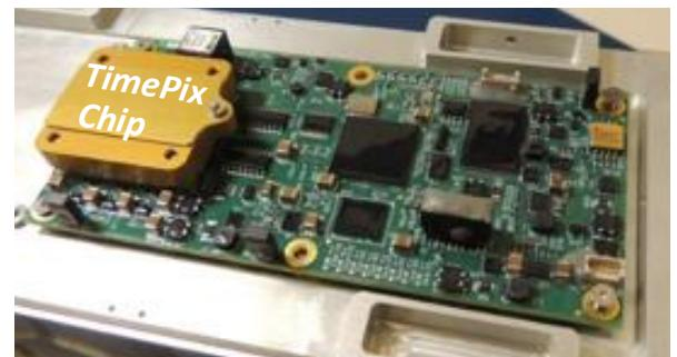
Single-Board Linear Energy Transfer (LET) Radiation Spectrometer
