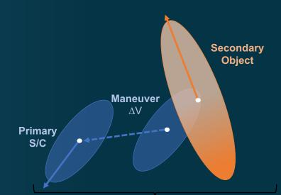
Primary S/C Collision Avoidance is the process of executing mitigative action, typically in the form of an orbital maneuver, to reduce collision risk.
