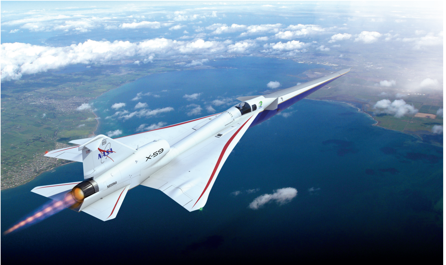
Figure 15–The X-59 Que斯特 is designed to fly supersonic without creating a sonic boom.
