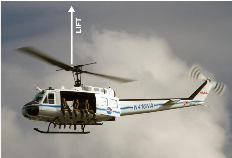
Figure 2. The blades on a helicopter create lift that moves it upward. Credit: NASA/ Dan Casper
