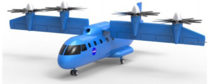
Figure 4. On some aircraft, the propellers can rotate to provide upward lift or forward thrust. Credit: NASA
