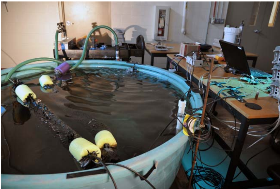
Figure 28 – a) Sediment-based microbial fuel cell in the Laboratory for Autonomous Systems Research (Credit: J. Hartman/NRL).
