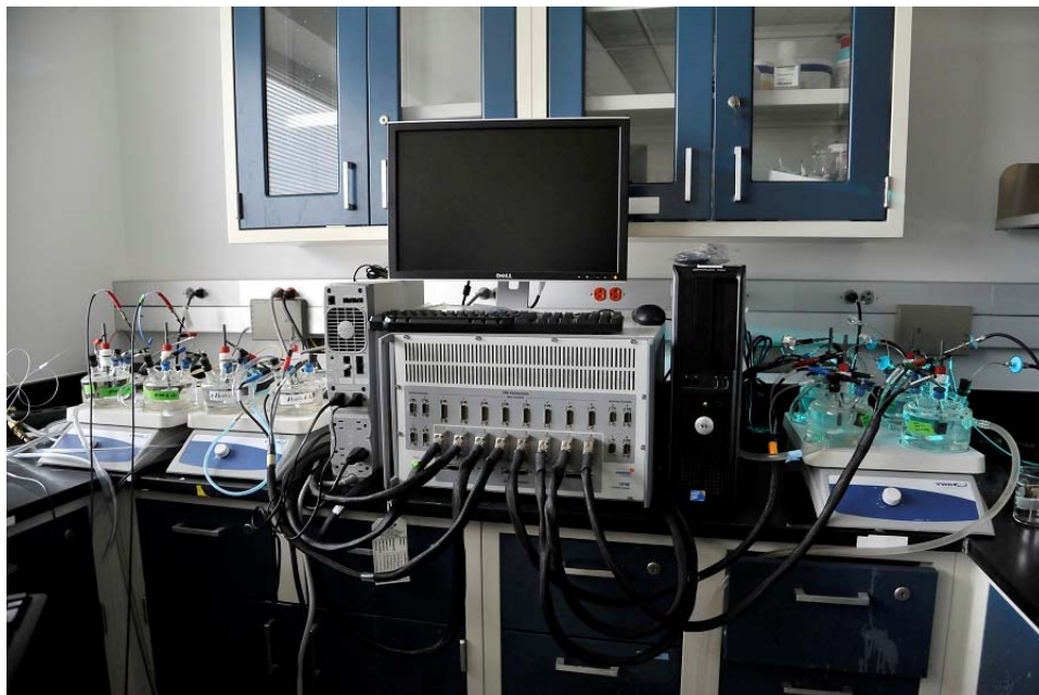
Figure 2 – This experimental instrumentation in the Laboratory for Microbial Electrochemistry one of five 8-channel potentiostats that can be used to simultaneously investigate performance of multiple bioelectrochemical systems. (Credit: J. Harman/NRL)
