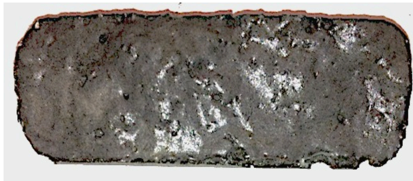
Figure 15. Plain regolith simulant sintered at 1100 °C for 1 hour
