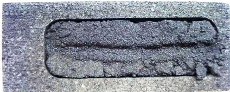
Figure 13. Plain regolith sintered at 975 °C for 1 hour
