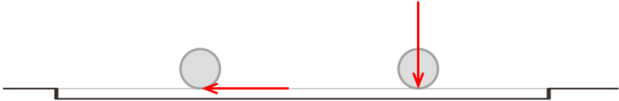
Figure 6: Roadway Boundary Conditions and Loading
