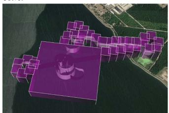
Fig. 12. Dynamic Operation Volume updates to remain in conformance
