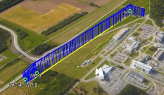
Fig. 2. BVLOS landing behind trees at a distance of 2,654 ft from launch point
