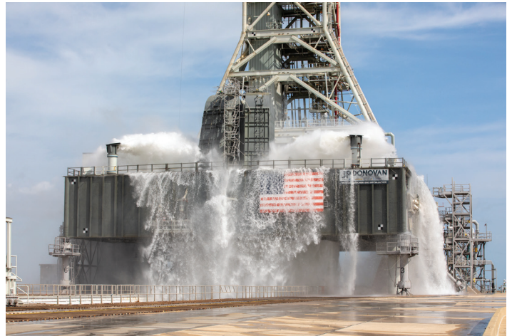
A wet flow test at Launch Pad 39B on September 13, 2019, tested the sound suppression system that will be used for launch of NASA’s Space Launch System for the Artemis I mission. During the test, about 450,000 gallons of water poured onto the Pad B flame deflector, the mobile launcher flame hole and onto the launcher’s blast deck. Photo credit: NASA/Kim Shifflett
