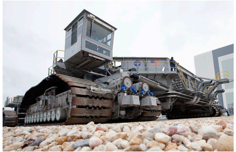
Above: Crawlerway rock is visible as NASA's upgraded crawler-transporter 2 (CT-2) returns to the Vehicle Assembly Building (VAB) at the agency's Kennedy Space Center in Florida from its trek to Launch Pad 39B. CT2's recently completed upgrades and modifications were tested to ensure the vehicle will be ready to support NASA's journey to Mars. Photo credit: NASA/Ben Smegelsky
