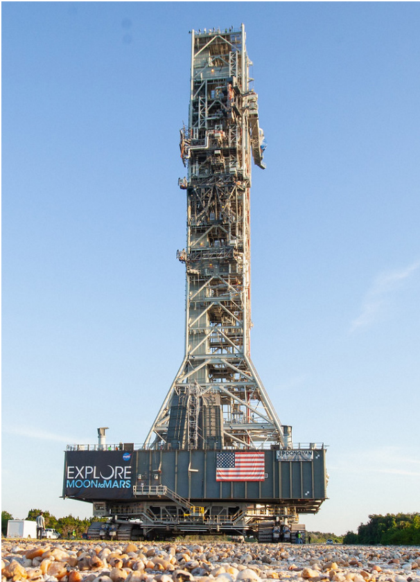
Above: Crawlerway rock is visible as NASA's upgraded crawler-transporter 2 (CT-2) returns to the Vehicle Assembly Building (VAB) at the agency's Kennedy Space Center in Florida from its trek to Launch Pad 39B. CT2's recently completed upgrades and modifications were tested to ensure the vehicle will be ready to support NASA's journey to Mars. Photo credit: NASA/Ben Smegelsky
