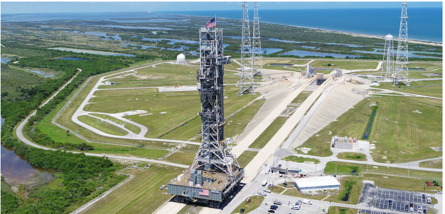
NASA's mobile launcher atop crawler-transporter 2 arrives at Launch Pad 39B on Aug. 31, 2018, at the agency's Kennedy Space Center in Florida for a fit check and systems testing. The 380-foot-tall mobile launcher is equipped with the crew access arm and several umbilicals that will provide power, environmental control, pneumatics, communication and electrical connections to NASA's Space Launch System and Orion spacecraft. Photo credit: NASA/Jamie Peer
