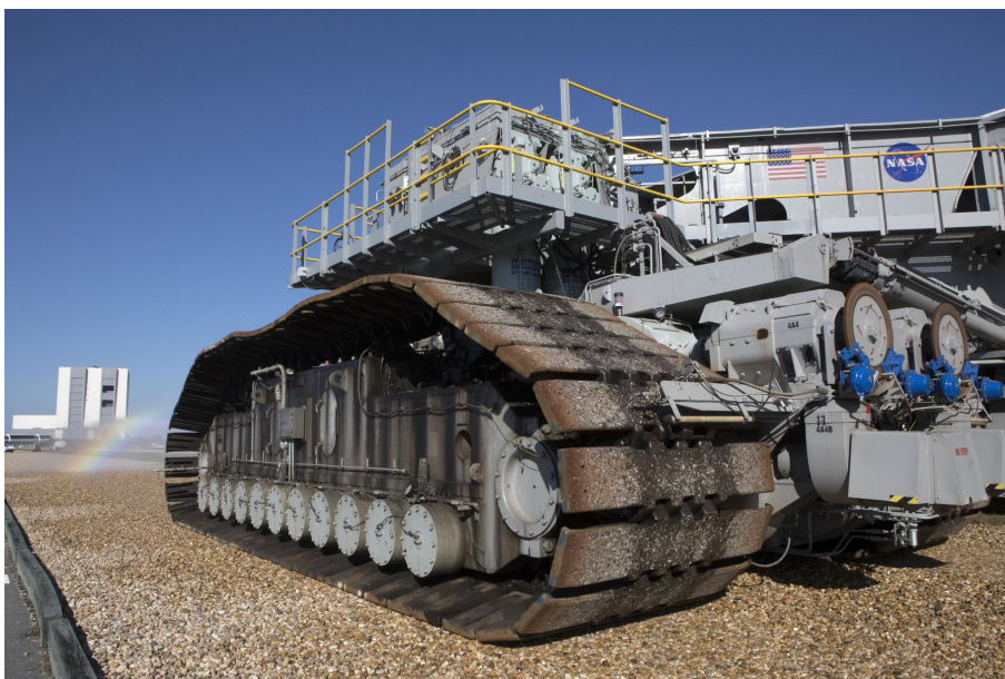
Crawler-transporter 2 (CT-2) moves slowly along the crawlerway on its way back to the Vehicle Assembly Building (in view in the background) at NASA's Kennedy Space Center in Florida. Water sprayed by a truck in front to reduce dust creates a small rainbow. The crawler took a trip to the Pad A/B split to test upgrades that will allow the giant vehicle to handle the load of the agency's Space Launch System rocket and Orion spacecraft atop the mobile launcher. Photo credit: NASA/Leif Heimbald
