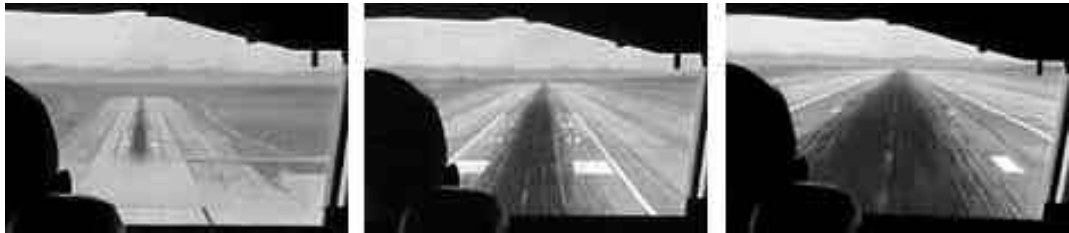
Figure 17. Pilot views of MD-11 performing a PCA Instrument Landing System-coupled approach and landing.
