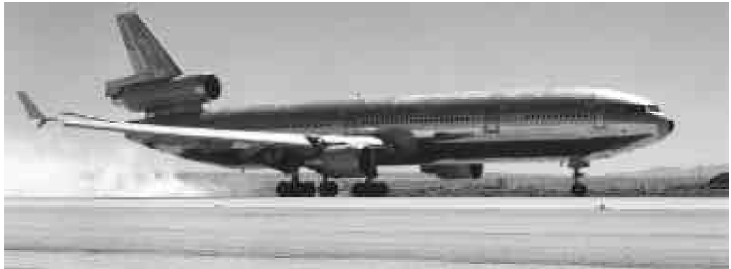
Figure 18. MD-11 touching down for the first time under engine power only, 11:38 a.m. August 29, 1995, at Edwards. (NASA photo EC95 43247-4 by Dennis Taylor).
