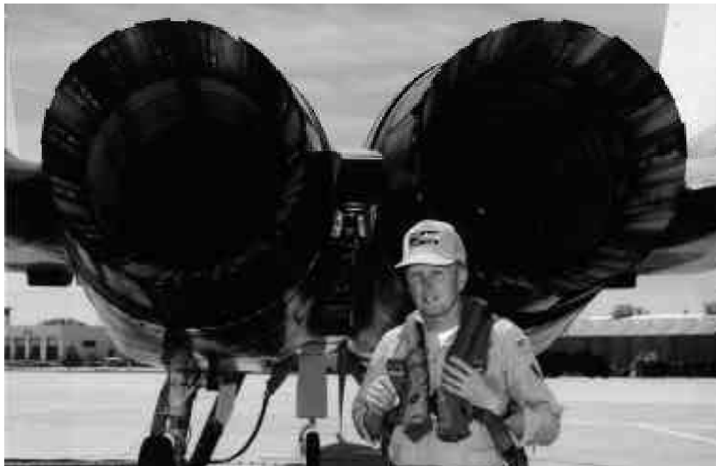
Figure 9. Gordon Fullerton and the two "brutes" (engines) in the F-15 after he had landed the aircraft using only engine power for control on 21 April 1993. (NASA photo EC93-41034-3 by Larry Sammons).
