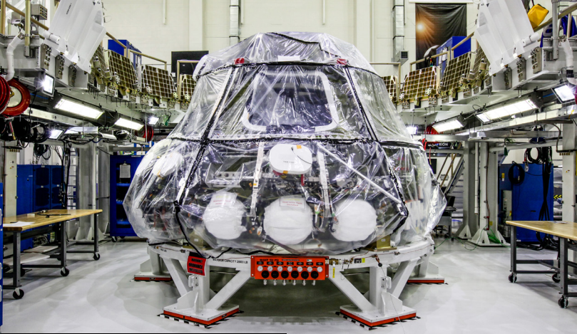
Crew Module Pressure Vessel Kennedy Space Center, Florida
