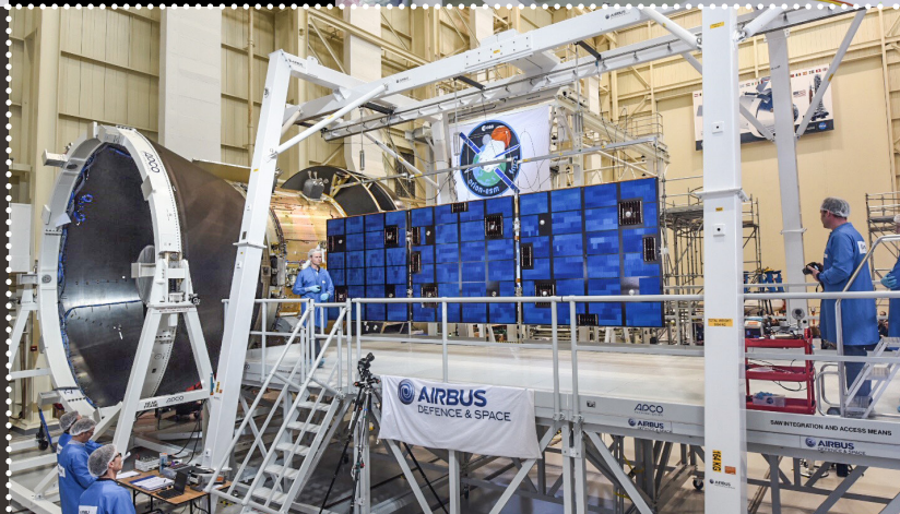
Service Module Structural Testing Space Power Facility at NASA Glenn Research Center's Neil A. Armstrong Test Facility
