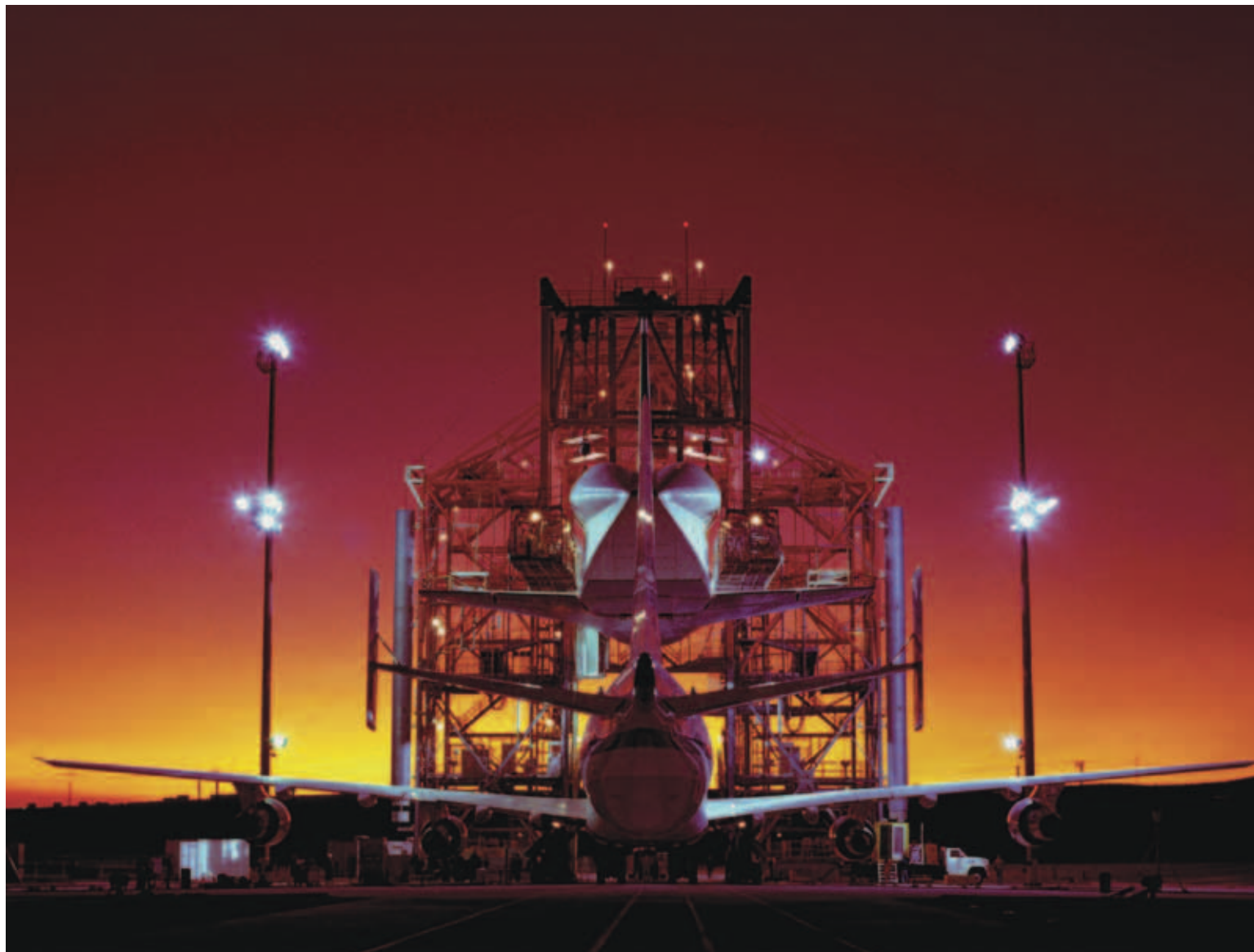
EC91 659-05 NASA Photo by Jim Ross Technicians begin preparations for Atlantis' attachment on the back of a 747 Shuttle Carrier Aircraft for the ferry flight back to Kennedy Space Center, Fla., following the STS-44 landing at Edwards in December 1991. Post-flight servicing of the orbiter and mating operations were carried out at Dryden in the Mate/Demate Device, the large gantry-like structure used in hoisting the spacecraft during post-spaceflight processing.
