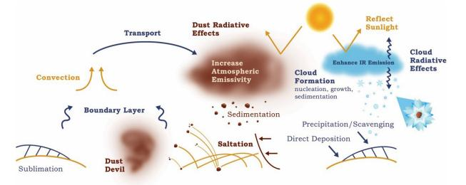
**Figure 1.1**: A depiction of the major processes influencing Mars' lower atmosphere. Each of these processes are handled within the NASA ARC Mars GCM. Most of these physical processes occur in other planets'/satellites' atmospheres as well.
