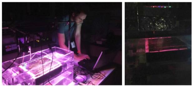
*Figure 3.6c*: Ames Pathway intern Owen Lehmer measuring O2 production in a microbial mat under (left) solar and (right) M dwarf spectral irradiance using a custom-designed LED array.
