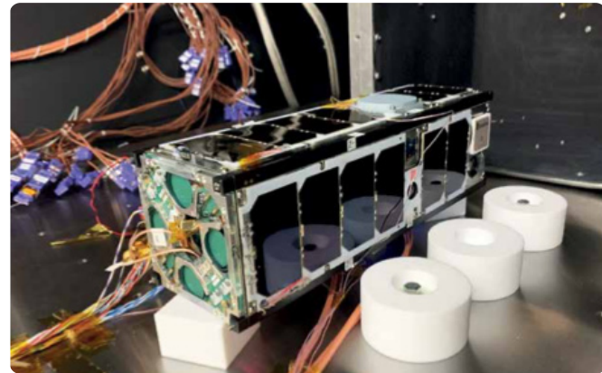
Neutron-1 is a 3-U CubeSat built by the Hawaii Space Flight Laboratory (HSFL) featuring an Arizona State University neutron detector that will be part of the Luna-H Map Mission to the Moon. Here, Neutron-1 is in HSFL's Thermal Vacuum Chamber.
