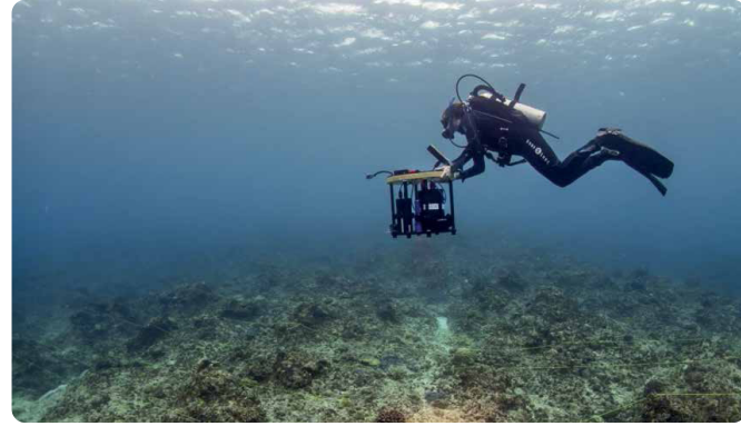
The DiveRay, an underwater instrument that captures hyperspectral reflectances from the benthos, in use at a coral reef off Guam. GEOCORE will use this data, along with other field-collected and satellite datasets, to characterize coral reef fish-spawning aggregation sites.
