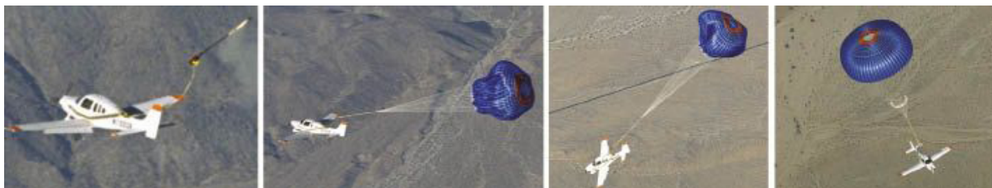
Figure 7- A parachute can deploy from a small airplane, allowing it to land safely even if its engine fails.
