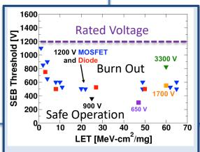
**Problem**: Silicon carbide power transistors work very well at high voltages on earth, but burn out due to radiation in space at voltages much lower than their rated voltage. Data points show the actual voltage at which devices burn out, versus the energy deposited by radiation.
