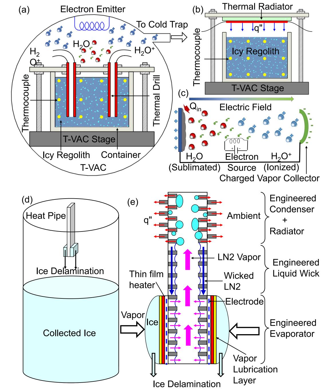
**Figure 1**: Advanced thermal mining technology: vapor extraction using (a) thermal drilling (b) radiative heating, (c) vapor ionization and transportation by electrostatic field, (d) ice re-capture in cold trap and (e) heat pipe surface engineering
