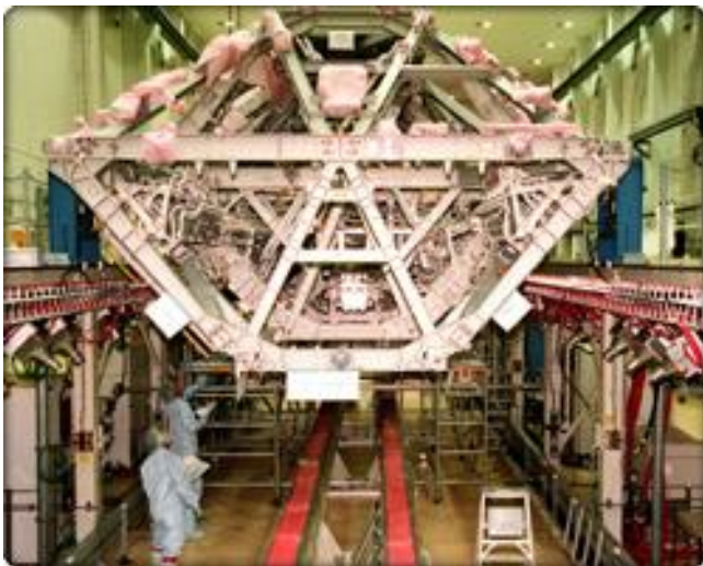
Figure 2. International Space Station Truss Segment cross section
