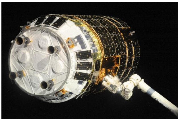
Figure 2. A close-up photograph of the Robotic Arm after it has grappled onto the HTV.
