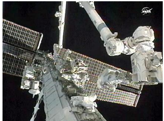
Figure 12. The Space Station Robotic Arm Grappler can also hold on to astronauts, using a different attachment
