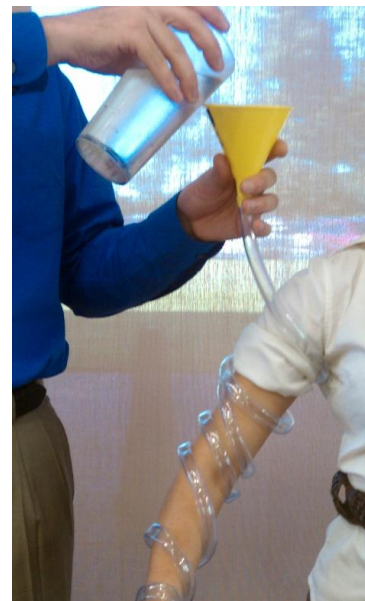
Figure 2. Cooling Loop made of clear plastic tubing and funnel.
