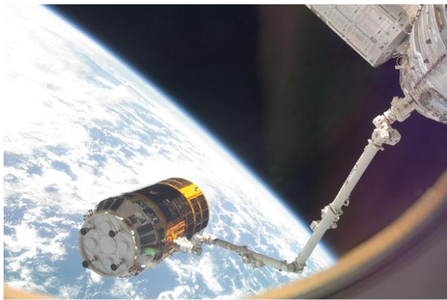
Figure 1. A photograph from a window of the International Space Station, showing the Robotic Arm grappling onto an 'H-2 Transfer Vehicle' or HTV.
