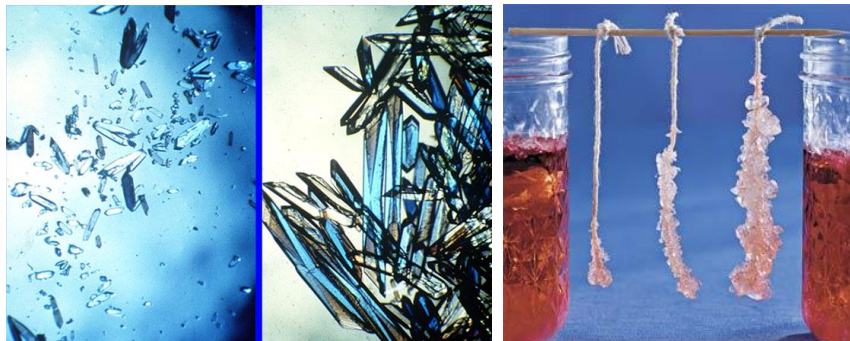
Figure 1. Insulin protein crystals grown (a) on earth and (b) on the ISS Laboratory. (c) Crystals grown in the classroom.
