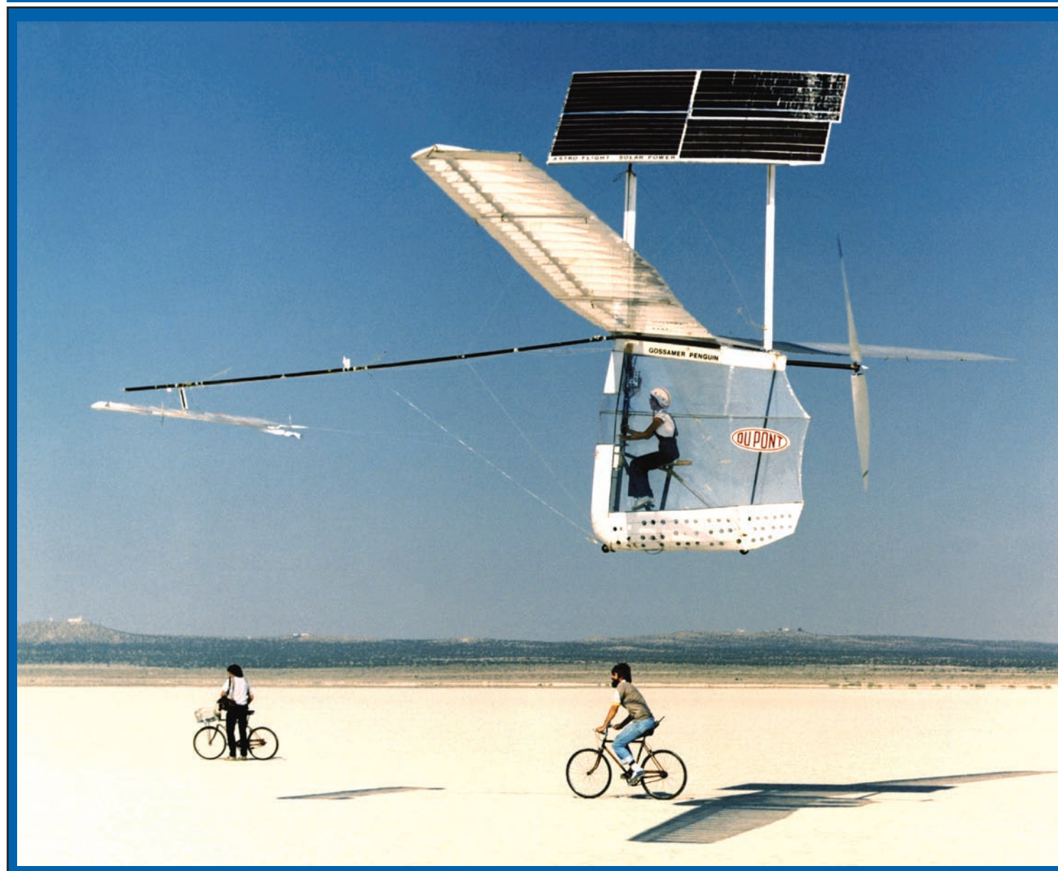
The solar-powered Gossamer Penguin flies on Rogers Dry Lake Bed during this flight on July 25, 1979. Ray Morgan, a Dryden consultant and former vice president of AeroVironment is chasing the Penguin by bicycle in the center of the image.
