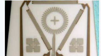
Microsensor for real-time monitoring within battery cells
