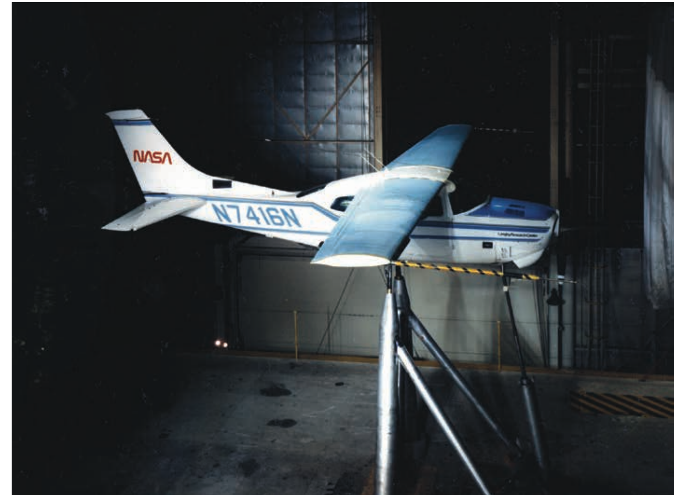
The Cessna 210 Centurion was tested at the NASA Langley Research Center in Hampton, Virginia, in the Langley 30-by-60-Foot Full Scale Tunnel in 1985 following the company's successful flight test program.
