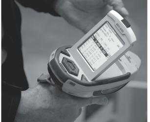
This material analyzer is one of the most recent tools used to uncover substandard materials and counterfeit parts.
