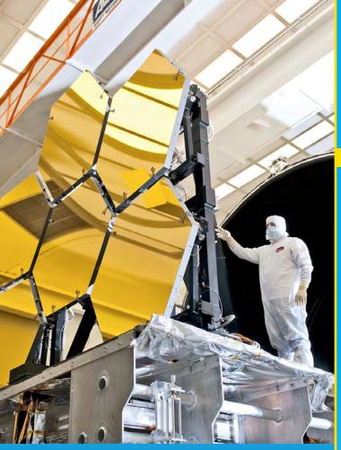
The first six James Webb Space Telescope's primary mirror segments are prepped to begin final cryogenic testing at NASA's Marshall Space Flight Center in Huntsville, AL.
