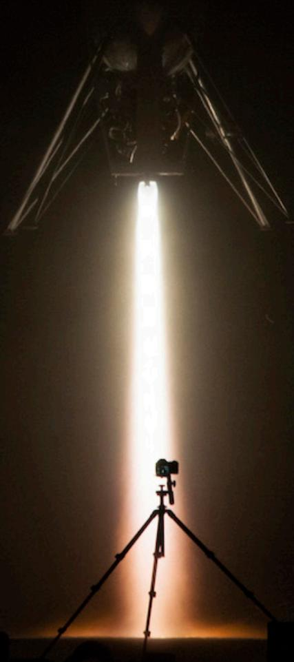
▷ August 25, 2015: Xaero-B, the new platform from Masten Space Systems, performs a tethered night flight to assess suitability of the platform for testing a starshade technology that would enable a future space mission to perform spectroscopy of Earth-like planets as far away as 60 light years (T0092). (Photo: NASA/Lauren Hughes)
