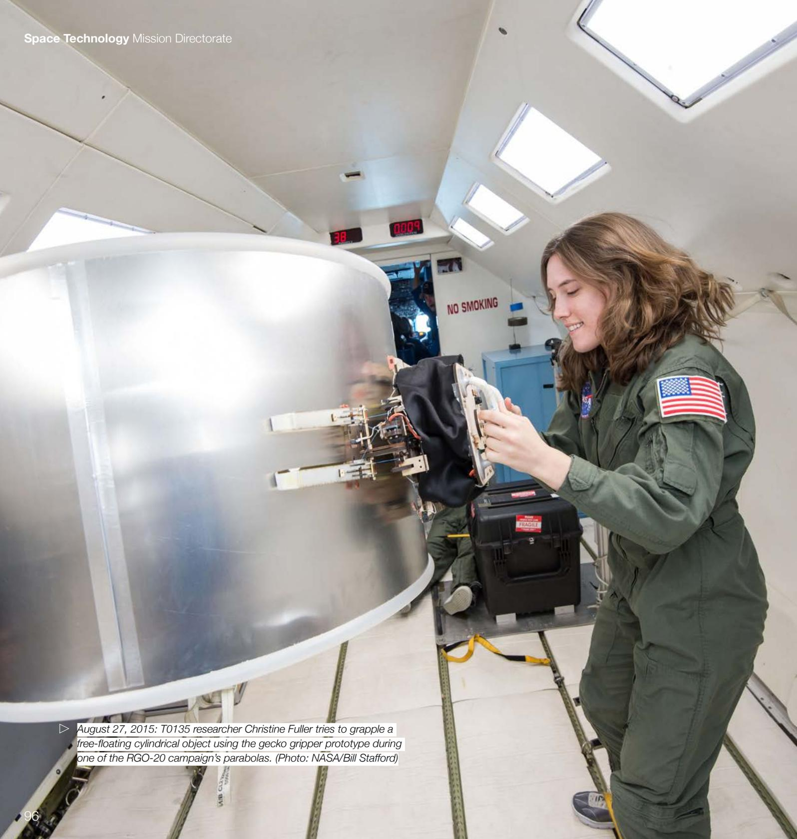
▷ August 27, 2015: T0135 researcher Christine Fuller tries to grapple a free-floating cylindrical object using the gecko gripper prototype during one of the RGO-20 campaign's parabolas. (Photo: NASA/Bill Stafford)
