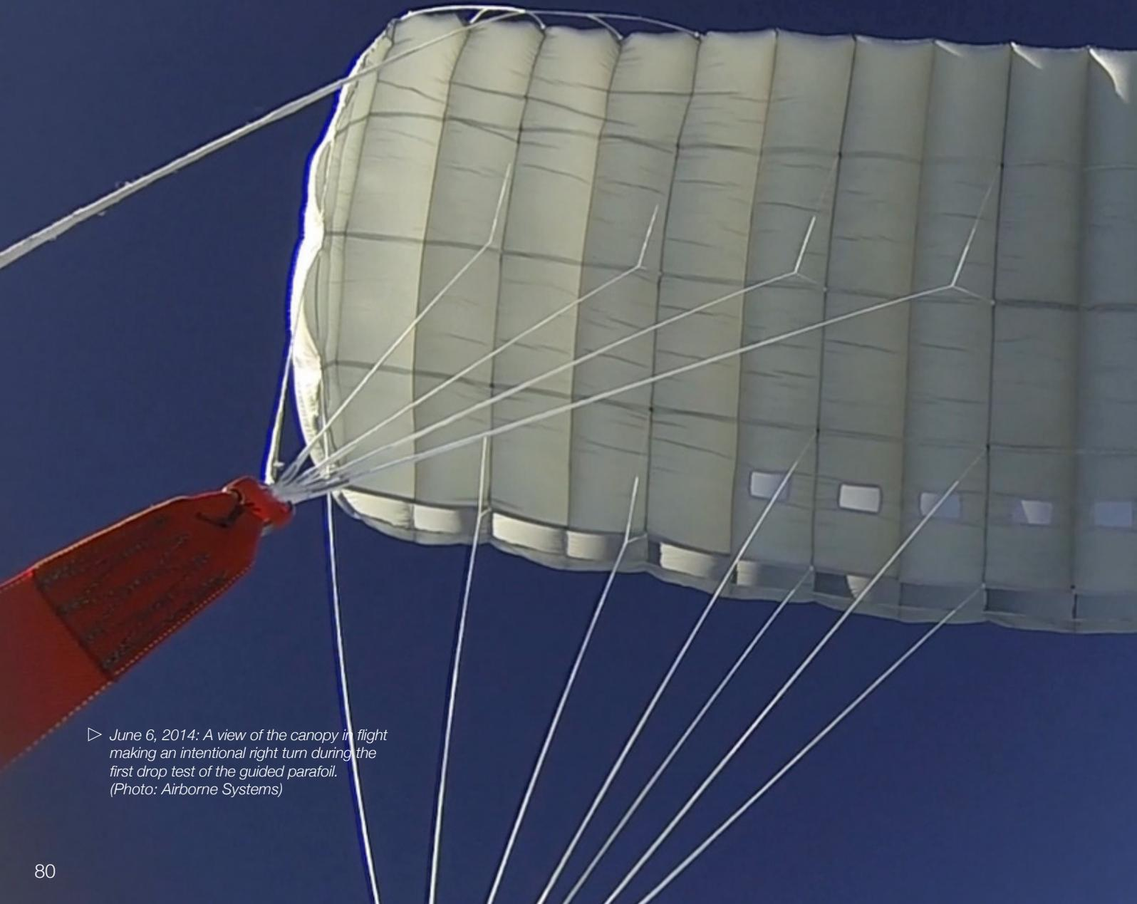
▷ June 6, 2014: A view of the canopy in flight making an intentional right turn during the first drop test of the guided parafoil. (Photo: Airborne Systems)
