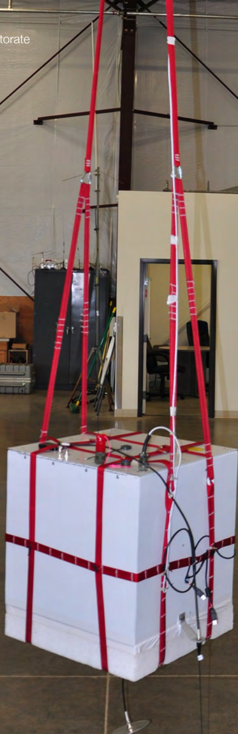
▷ October 11, 2013: Payload hang test with the TAMLACE payload inside the Small Balloon System (SBS) gondola. The 1090ES ADS-B transponder antenna can be seen underneath the gondola. It is suspended 6 feet below the gondola during flight. (Photo: Near Space Corporation)
