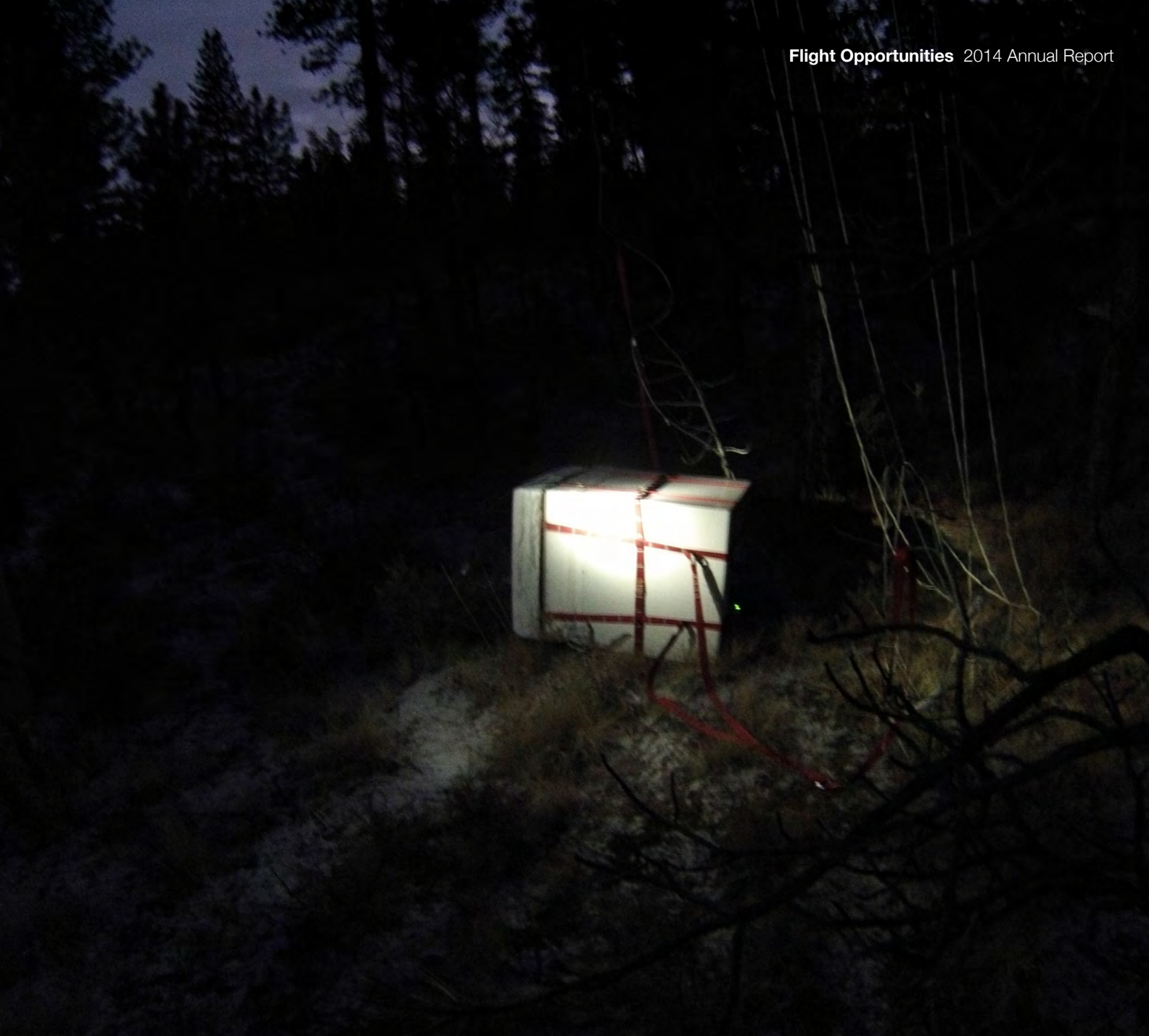
▷ December 5, 2013: post-landing recovery of the Small Balloon System (SBS) gondola carrying the TAMLACE payload testing reception of the surrogate Satellite-based ADS-B. (Photo: Near Space Corporation)
