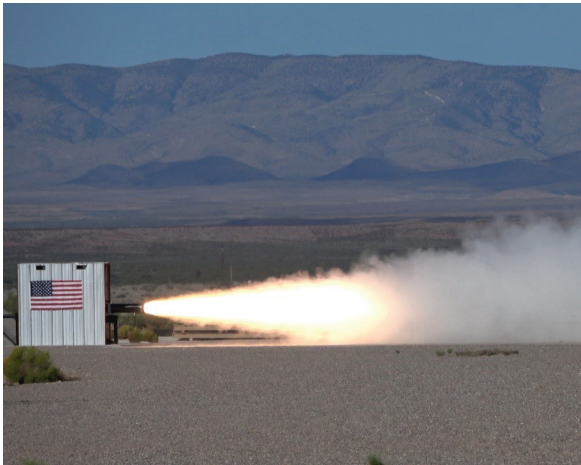
Researchers conduct a rocket motor qualification test at the Space Propulsion Center, Spaceport America, New Mexico. Credit: UP Aerospace
