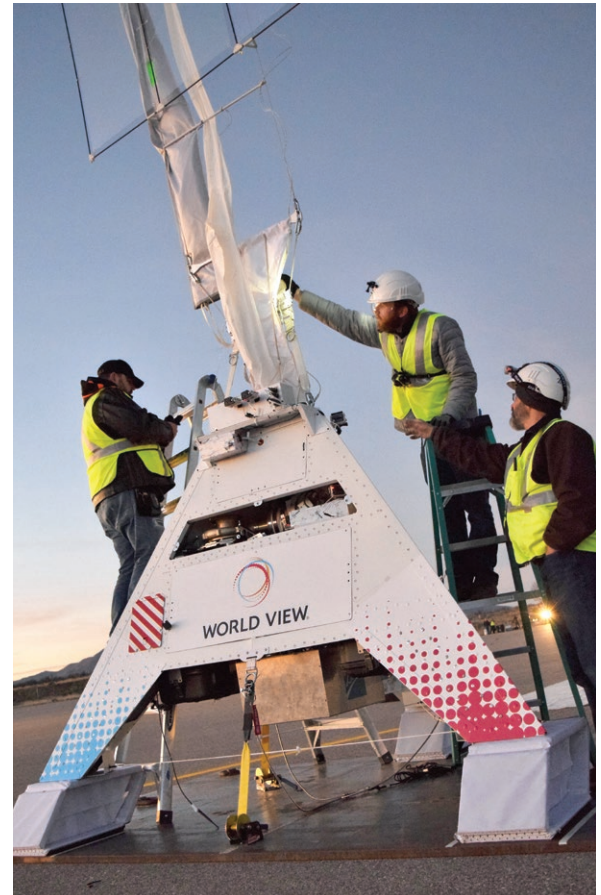
World View personnel prepare their advanced altitude control technology for a flight test on the Stratollite high-altitude balloon system. Credit: World View Enterprises
