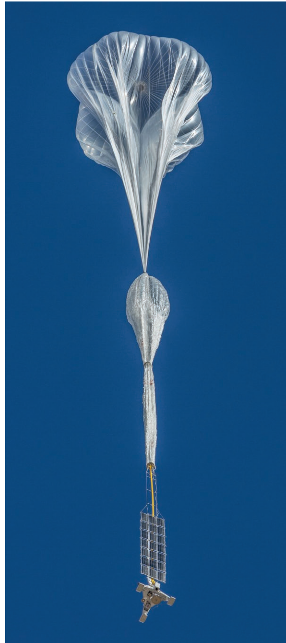
The Stratollite high-altitude balloon system. Credit: World View Enterprises
