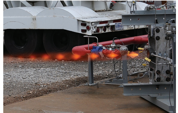
Dynetics performs an engine hot-fire test at NASA's Marshall Space Flight Center using peroxide/kerosene propellant. Credit: NASA
