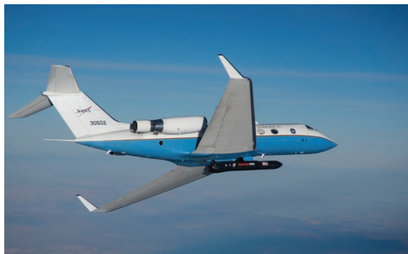
NASA's C-20A undergoes a flight test with Generation Orbit's hypersonic pod attached. Credit: NASA
