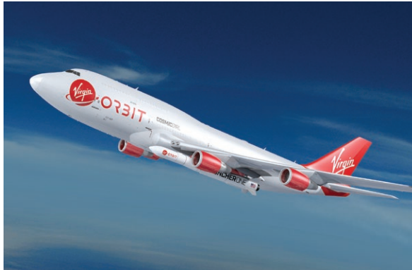
LauncherOne is shown being carried by Virgin Orbit's Cosmic Girl carrier aircraft. Credit: Virgin Orbit
