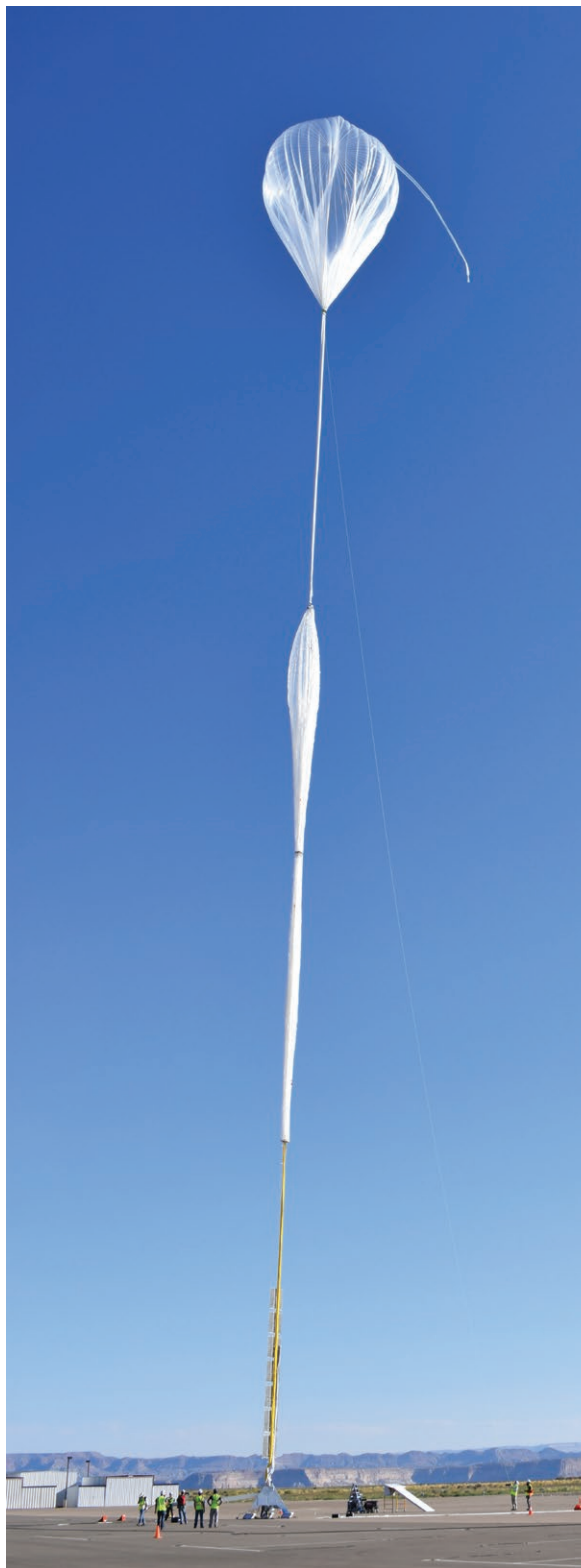
The World View Stratollite is shown here in its stand-up configuration prior to launch. Credit: World View Enterprises
