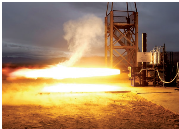
A 3D-printed injector from NASA's Marshall Space Flight Center is hot-fire tested by Vector using liquid oxygen/propylene propellant. Credit: Vector Space Systems
