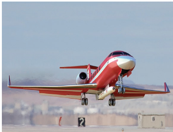
GOLauncher 1 is an air-launched single-stage rocket under development to serve microgravity, astrophysics, and hypersonics researchers. Photo credit: Generation Orbit
