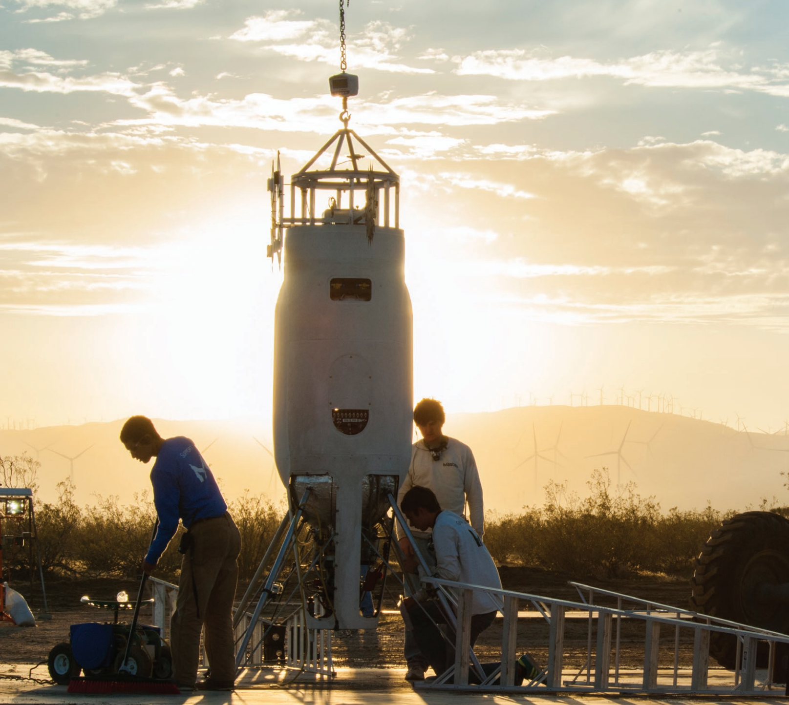
Teams from the University of Colorado Boulder and Masten Space Systems flew a set of tethered flights with a 26-inch starshade mounted to the Xaero vehicle. The campaign investigated using Masten Space Systems' vertical takeoff, vertical landing rocket as a stable platform to conduct high-contrast astronomy with an external occulter. Photo credit: NASA
