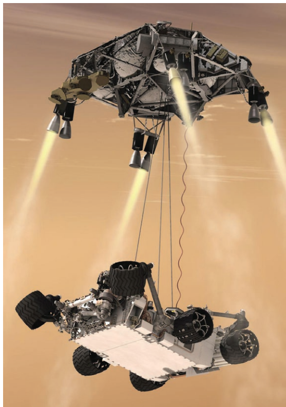
An artist's concept of the 2012 Mars Curiosity Landing. Mars 2020 will use a nearly identical landing system but with added precision from the Lander Vision System.
