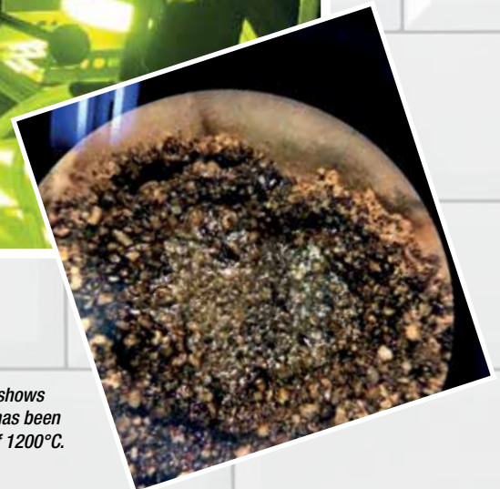
In our laboratory at the University of Maine, we have built a test stand where we can sinter samples of simulated lunar soil using concentrated light that mimics concentrated sunlight.
