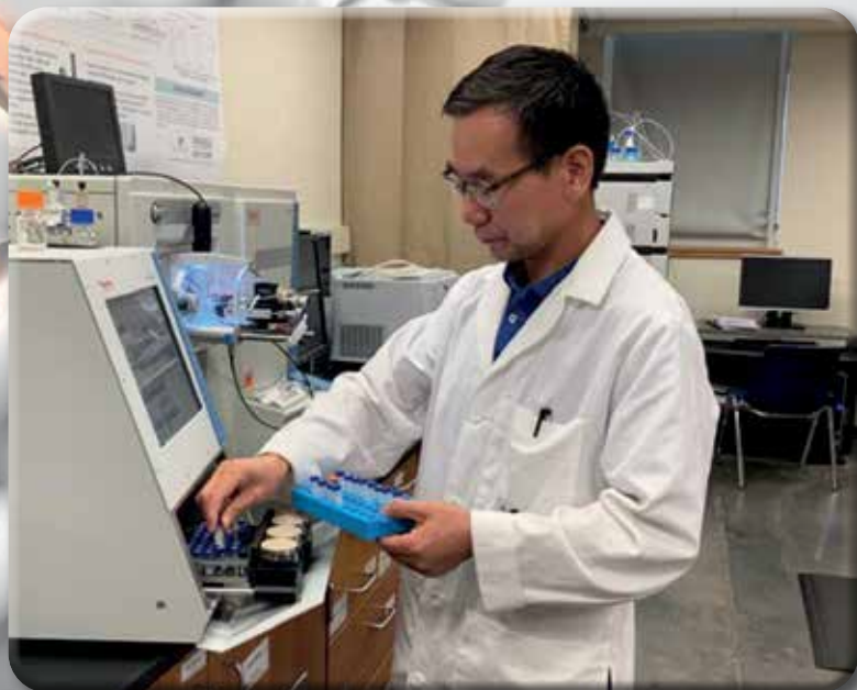
Liquid chromatography-mass spectrometry (LC-MS)-based proteomics was used in this project to quantify the global changes of protein expression levels in MSCs under simulated microgravity. Proteins were extracted from cells and processed for LC-MS analysis. In the photo, Dr. Xinzhu Pu was loading the samples on the LC-MS instruments for analysis.
