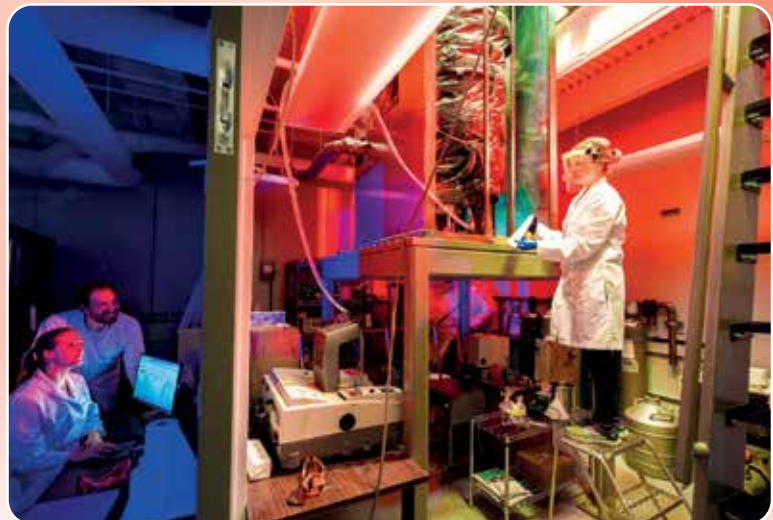
View of the Andromeda simulation chamber, used to test materials under Titan surface conditions (left: Kendra Farnsworth and Vincent Chevrier, right: Ellen Czaplinski). The W.M. Keck Laboratory for Space and Planetary Simulations at the University of Arkansas hosts several simulation chambers used to study planetary environments.
