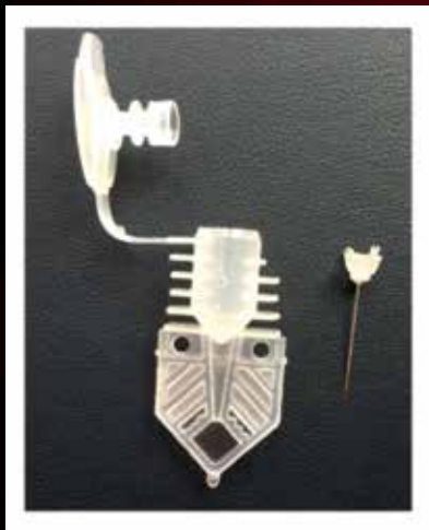
The RNA capture pins interface elegantly with the COTS reaction tubes. The pins are functionalized with capture thymine nucleobases. The RNA capture pin is punctured into biological tissue, the RNA tail attaches to the pin, and is collected for analysis by simply removing the pin from the tissue.
