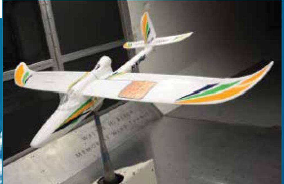
WSU's wind tunnel test of the SANSEC sensor for wing shape sensing.
