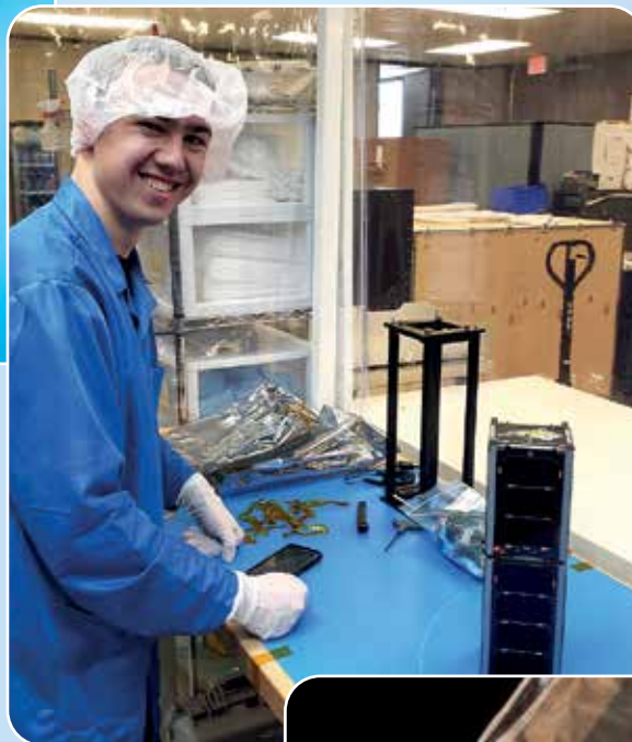
RadSat-u from Montana State University tests a new computer architecture that can recover from faults caused by space radiation on its core+memory blocks.
