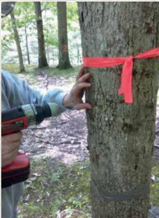
The probe is inserted into the sapwood at a depth of 30 mm using a drill bit and covered with a reflective bubble wrap for insulation.
