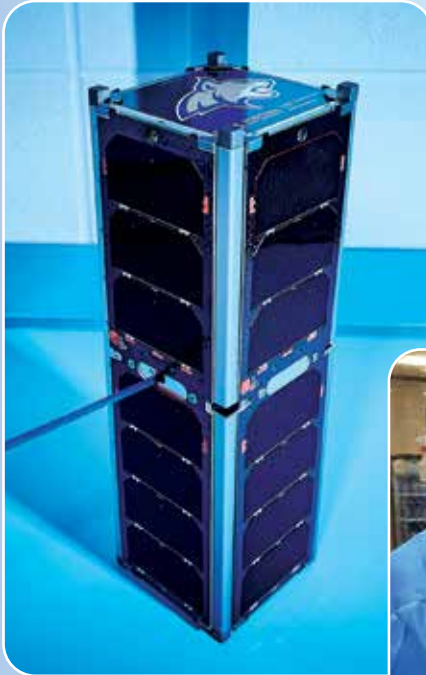
RadSat-u from Montana State University tests a new computer architecture that can recover from faults caused by space radiation on its core+memory blocks.
