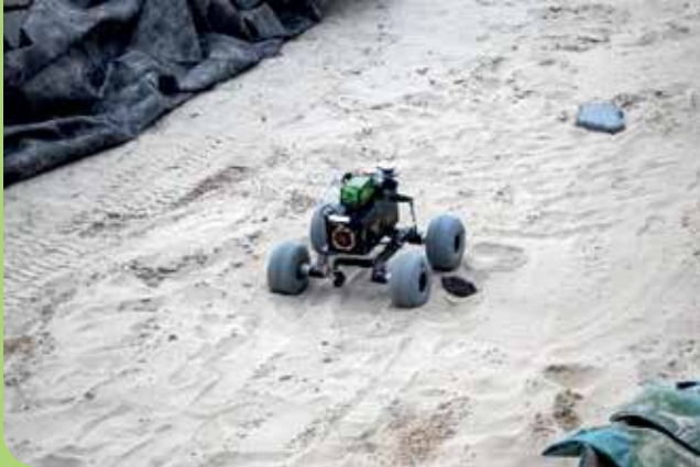
(Left) A Pathfinder robot experiencing slippage due to the slope and sandy terrain in JPL Mars Yard; (Right) another Pathfinder collecting data in a Utah desert.
