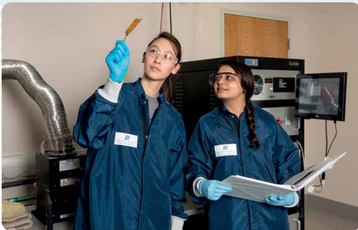
Dr. Courtney Hollar (left) and Twinkle Pandhi (right) inspect an array of flexible carbon nanotube sensors printed on polyimide substrate
