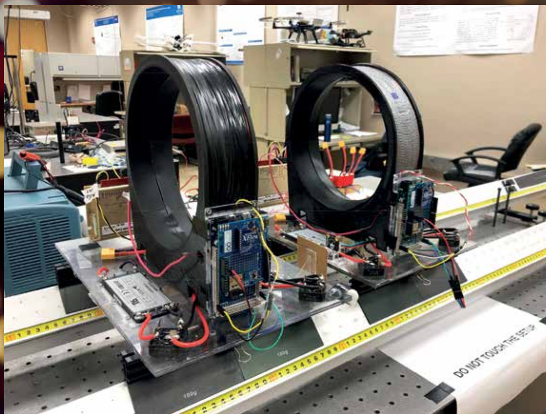
Electromagnetic formation-flying satellite experiment: Electromagnetic actuators (experimental setup pictured) are used to control the relative position and attitude of small satellite swarms
