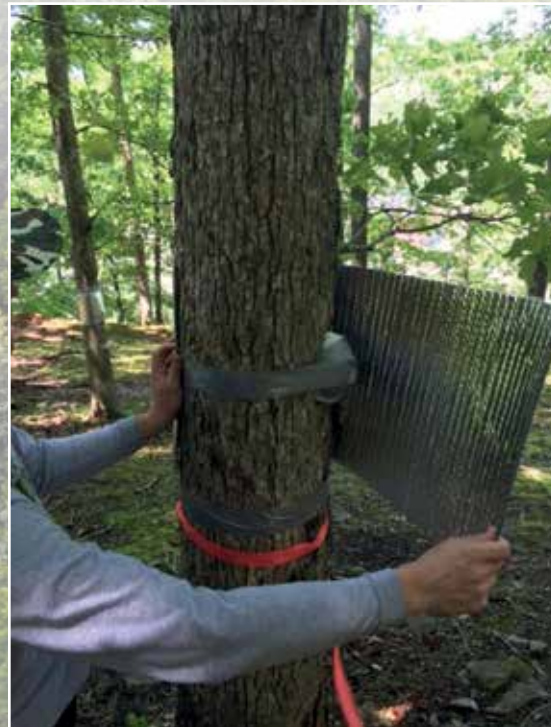
The probe is inserted into the sapwood at a depth of 30 mm using a drill bit and covered with a reflective bubble wrap for insulation.
