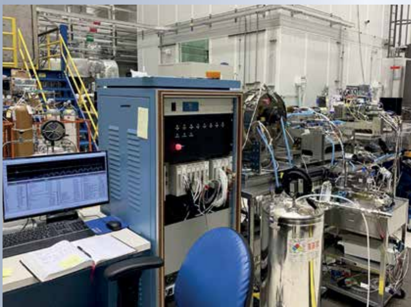
ISS water reclamation assembly unit duplicate at MSFC.
