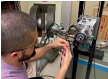
Connecting magnetic field coils on the cold-head of the cryo-stat.
