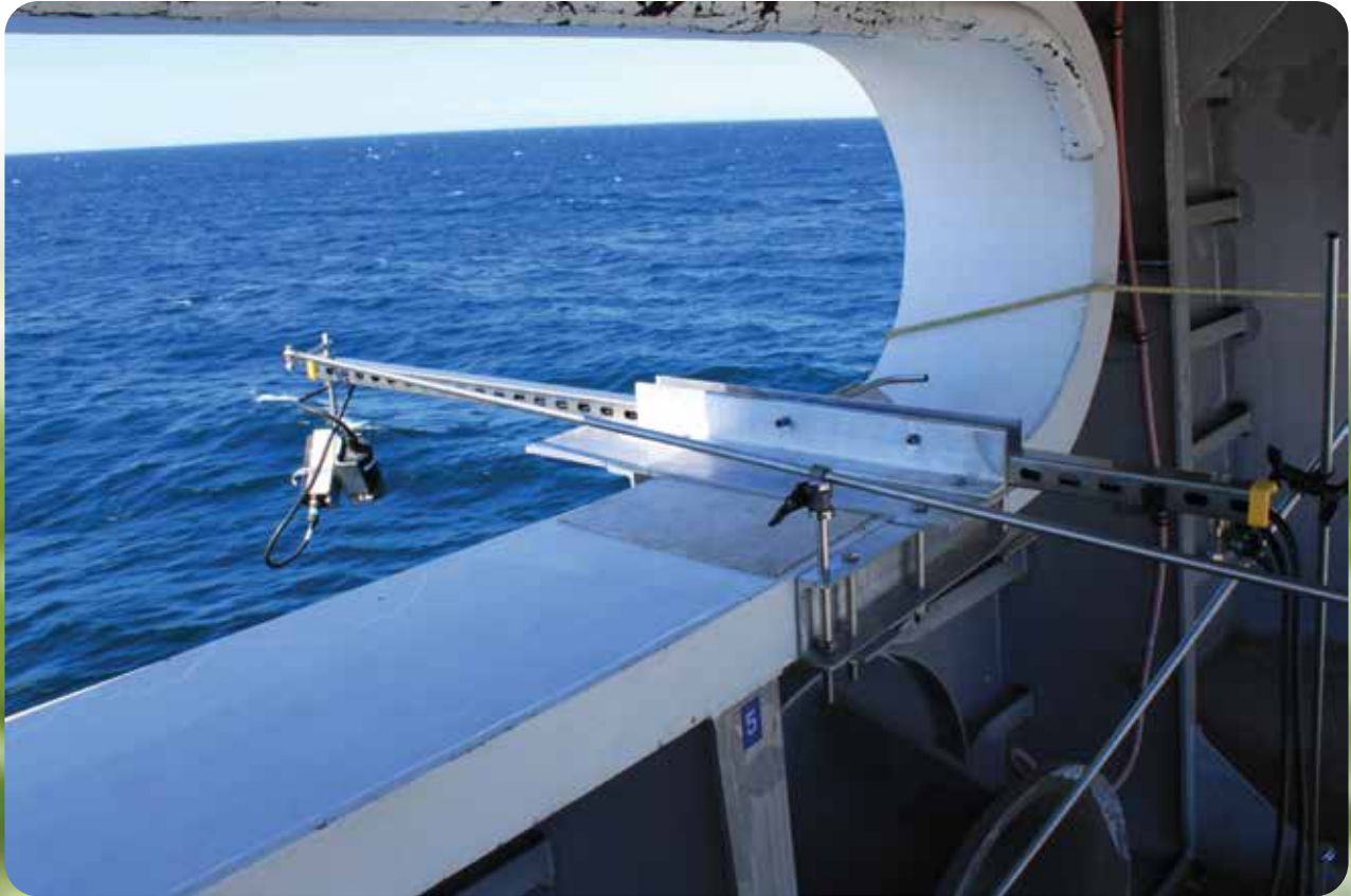
The hyperspectral ocean optical sampling instrument HyperSAS mounted on the bow of the ferry "The Cat" crossing the Gulf of Maine in summer 2018.
