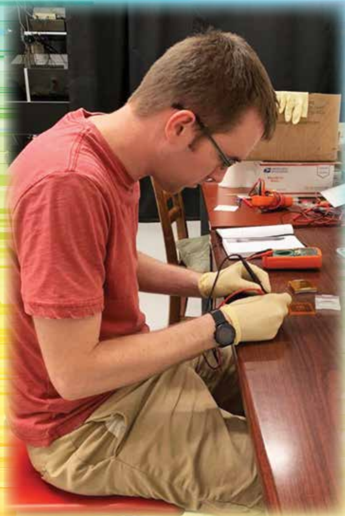
Graduate student probing the electrical properties of solar cells prior to analysis under space conditions
