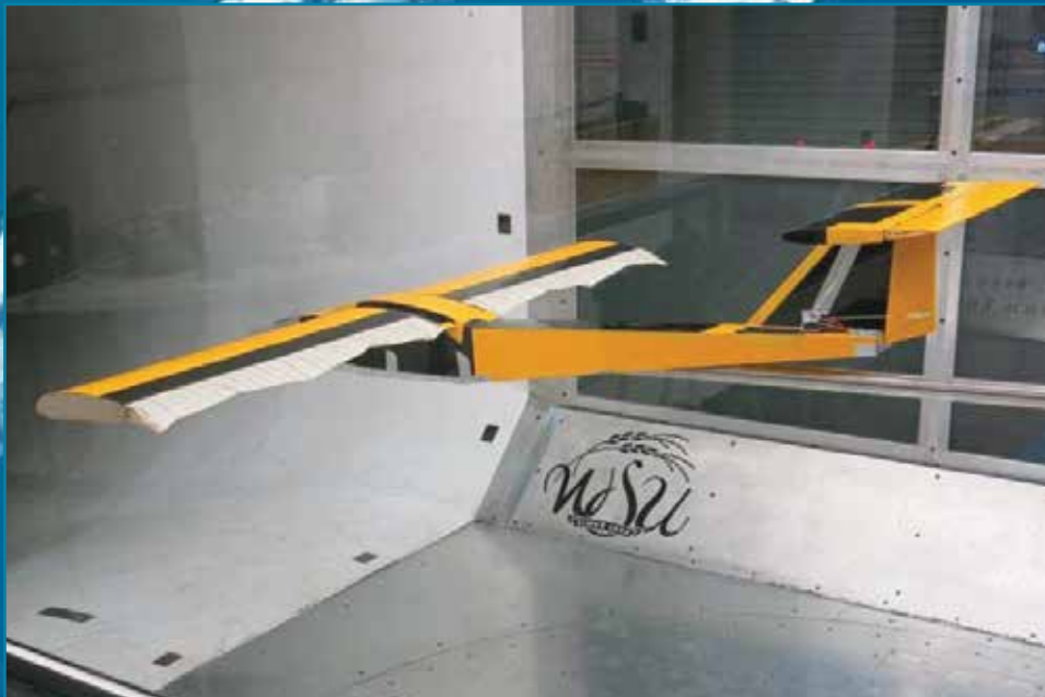
WSU's wind tunnel test of a Variable Camber Continuous Trailing Edge and Flaps (VCCTEF) aircraft.
