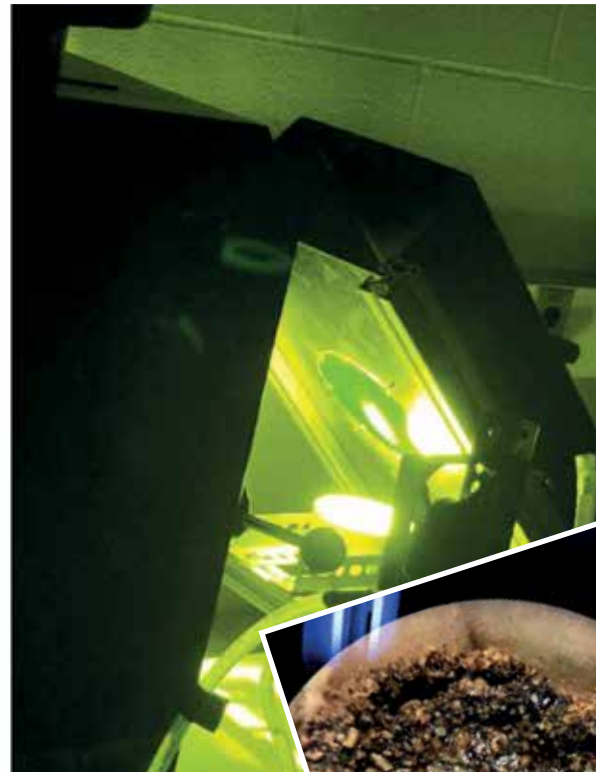
In our laboratory at the University of Maine, we have built a test stand where we can sinter samples of simulated lunar soil using concentrated light that mimics concentrated sunlight.
