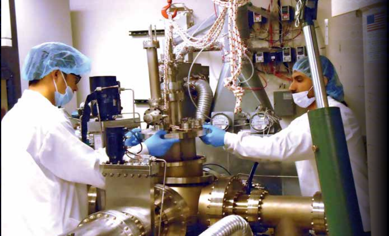
The researchers at the University of Arkansas Fayetteville (UAF) are working on the material growth using ultra-high-vacuum chemical vapor deposition (UHV-CVD) equipment located at Engineering Research Center at UAF campus.
