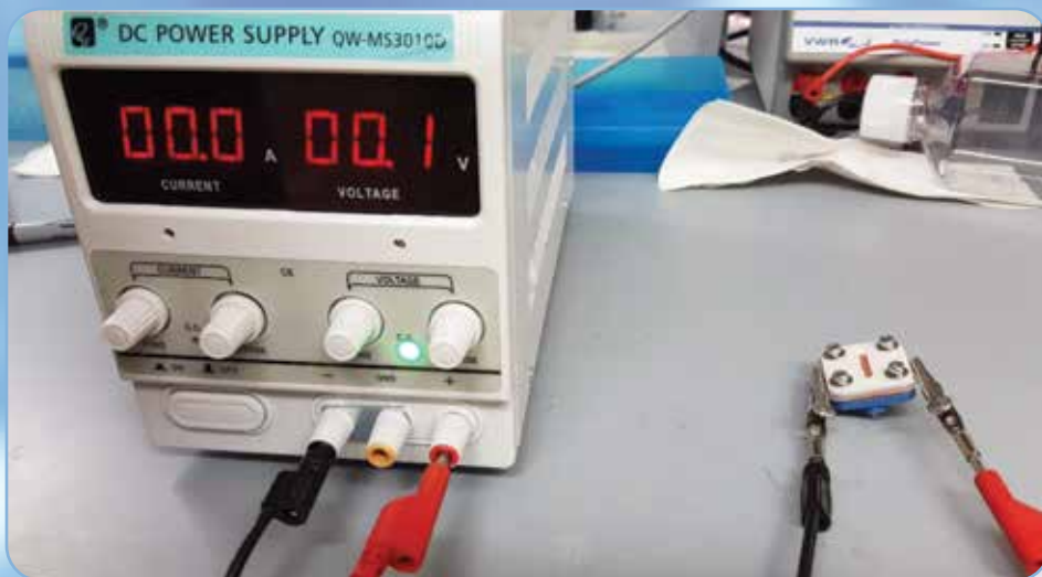
Photo 1: Miniaturized Vertical Comet Assay device in testing. Only 0.1 V is necessary to perform electrophoresis in this device for about 90 minutes to extract detectable broken DNA strands, as compared to the traditional electrophoresis at the tens voltage level for a few hours.
