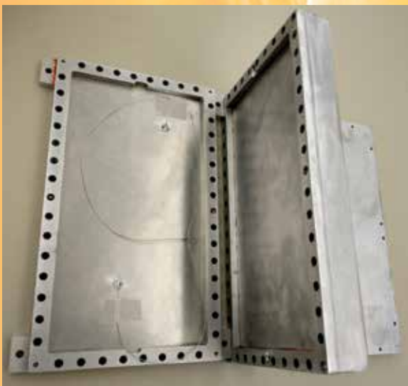
New Mexico Tech ISS payload carrying SHM LEO experiments. (a) top section with sensor layout for guided wave experiment, (b) bottom plate with electronic hardware for SHM experiments.
