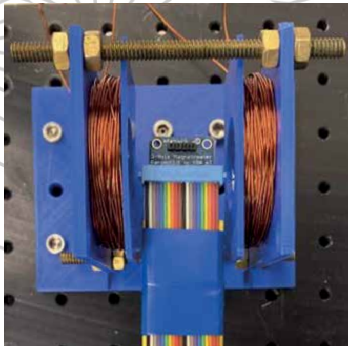
Helmholtz coils to apply precise magnetic field and calibrate with room temperature magnetic sensor.
