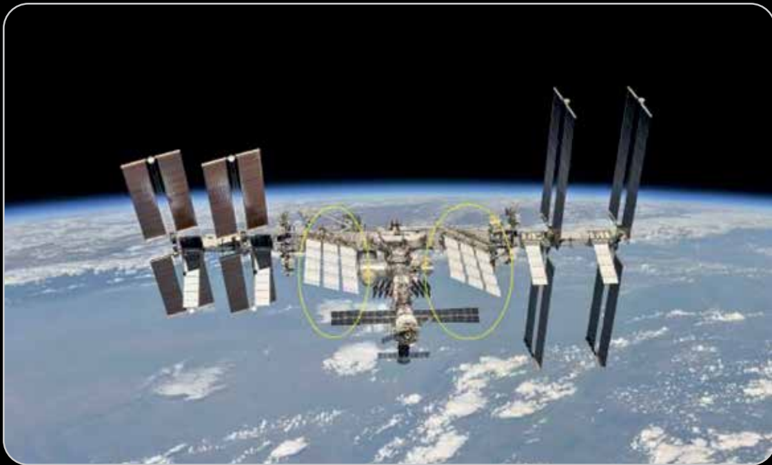
Figure 1: The External Ammonia Coolant Loops portion of the External Active Thermal Control Subsystem (EATCS) on the ISS are circled above. Photo Credit: NASA
