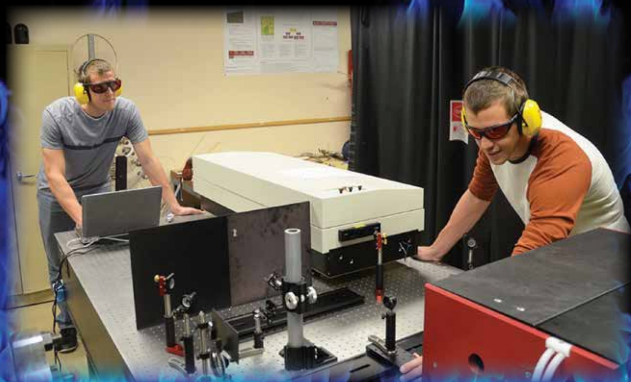
University of Wyoming graduate students conduct formaldehyde planar laser induced fluorescence experiments to visualize cool flame structures
