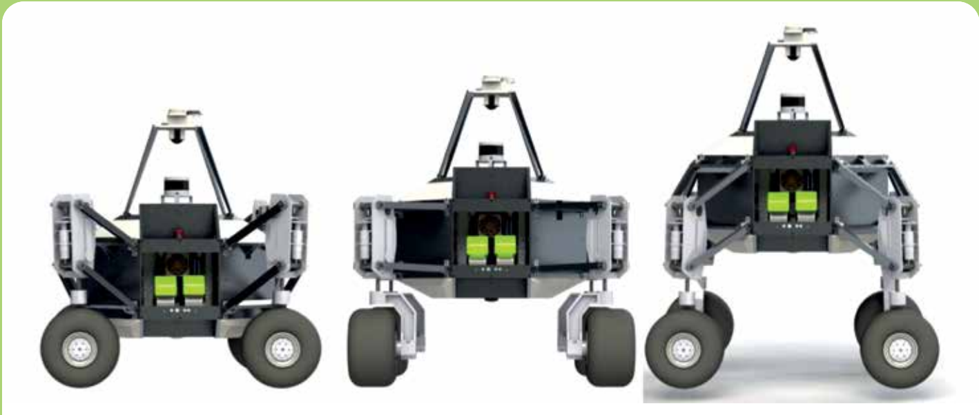
The design of the Fast Traverse Rover at its minimum (left, 15 cm), cruise (middle, 30 cm), and maximum (right, 45 cm) ground clearance points.
