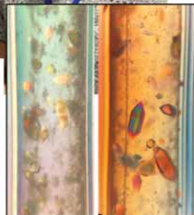
Earth-grown crystals (left) vs. microgravity-grown crystals (right) from the same crystallization conditions.
