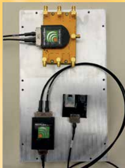
New Mexico Tech ISS payload carrying SHM LEO experiments. (a) top section with sensor layout for guided wave experiment, (b) bottom plate with electronic hardware for SHM experiments.
