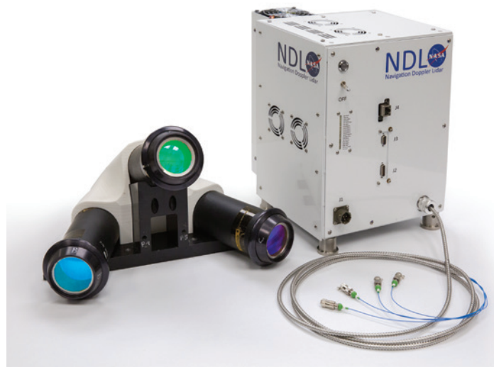
Langley’s NDL uses lasers that bounce off the ground and back to the instrument, providing velocity and range information upon approach for landing on the Moon. Credits: NASA/David C. Bowman
