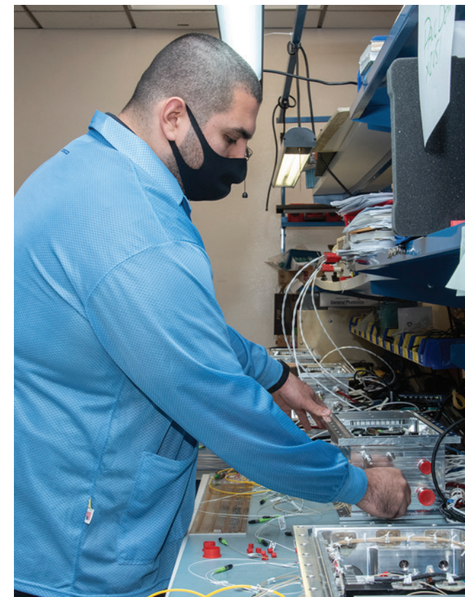
A project from Armstrong will investigate the viability of a ground-proven system for collecting strain and temperature measurements for space-based applications. Here, NASA research engineer Jonathan Lopez prepares a compact version of the system, known as a FOSS rocket box. Credits: NASA
