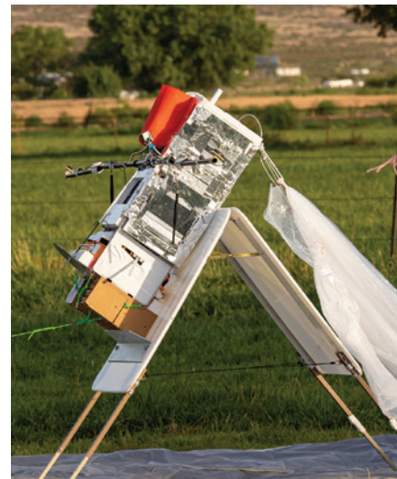
Instruments that may help advance infrasound investigations on Venus and other planets are launched on a Raven Aerostar high-altitude balloon in July 2020. Credits: Sandia National Laboratories
