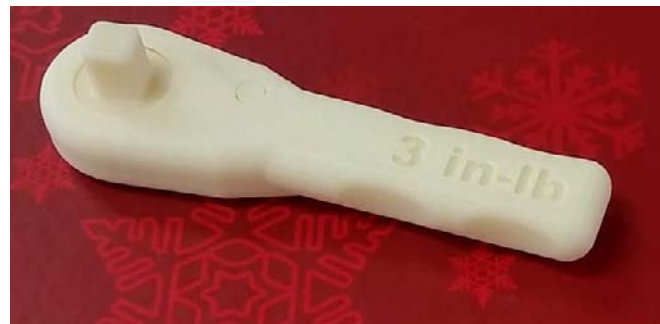
The 3D printer on the space station allows astronauts to print materials when needed. The first ratchet wrench printed aboard the space station was designed on Earth, then sent as a file to the station and printed on the 3D printer in 2014.
