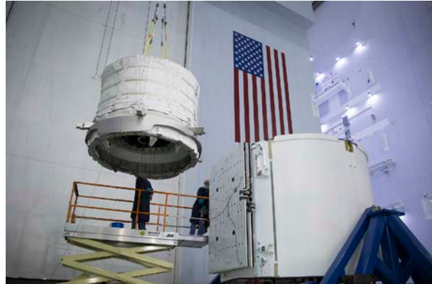
The Bigelow Expandable Activity Module (BEAM), developed for NASA by Bigelow Aerospace, is lifted into SpaceX's Dragon spacecraft for transport to the International Space Station.
