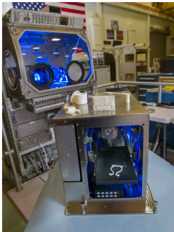
The 3D printer on the space station allows astronauts to print materials when needed. The first ratchet wrench printed aboard the space station was designed on Earth, then sent as a file to the station and printed on the 3D printer in 2014.
