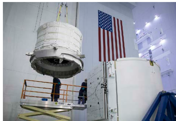
The Bigelow Expandable Activity Module (BEAM), developed for NASA by Bigelow Aerospace, is lifted into SpaceX's Dragon spacecraft for transport to the International Space Station.
