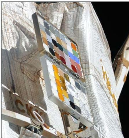
Figure 20. Russian Replaceable Cassette-Container on the Russian Service Module.
