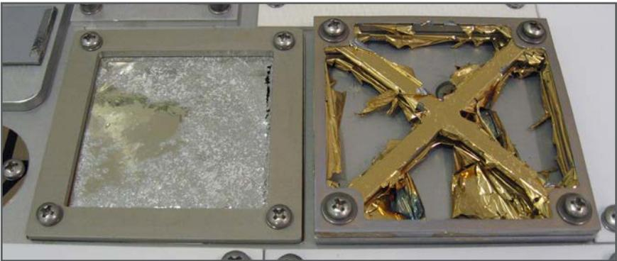
*Figure 6. Postflight photograph displays thin film samples from the Materials International Space Station Experiment-4 with catastrophic failure of both coatings related to combined thermal cycling and atomic oxygen erosion.*
