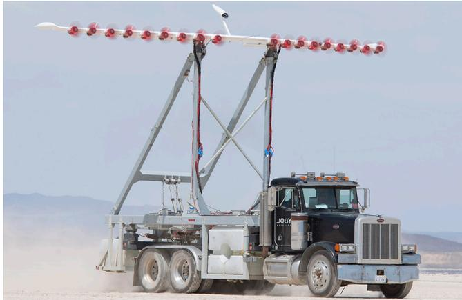
The integrated experimental testbed reached speeds of up to 73 mph in data collection to create the effect of a wind tunnel on the ground. (NASA Photo/Tom Tschida)
