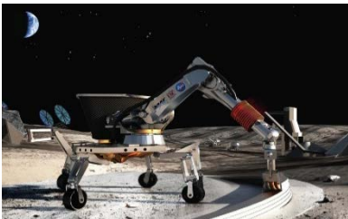
Illustration of a contour crafting robot building a structure out of processed lunar soil.
