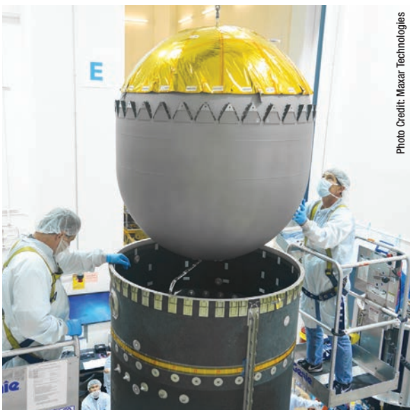
The fuel tank that On-Orbit Servicing, Assembly and Manufacturing Mission 1 will use to refuel Landsat 7 and potentially other satellites is completed at a Maxar Technologies facility.
