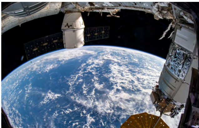
The Northrop Grumman Cygnus (right foreground), and the SpaceX Dragon (top rear) cargo vehicles are seen attached to the orbiting laboratory. Commercial resupply missions regularly bring new science and cargo to the space station. Credit: NASA
