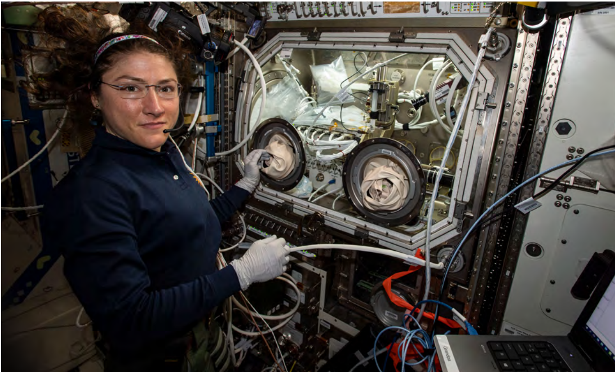
NASA astronaut Christina Koch performs science operations in the Microgravity Science Glovebox for the Ring Sheared Drop investigation into the mechanisms of Alzheimer's. Koch set a record for the longest single spaceflight in history by a woman, after 328 days living and working aboard the International Space Station. Her extended mission will provide researchers the opportunity to observe effects of long-duration spaceflight on a woman. Credit: NASA
