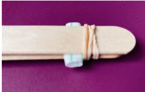
Figure 5. Wrap one of the thin rubber band around the tongue depressors to hold them together
