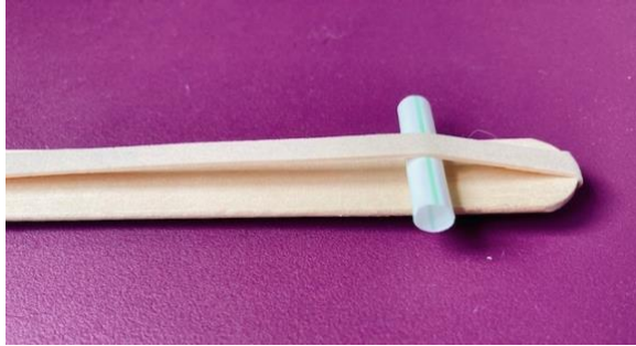
Figure 3. Place one piece of the straw between the rubber band and the tongue depressor
