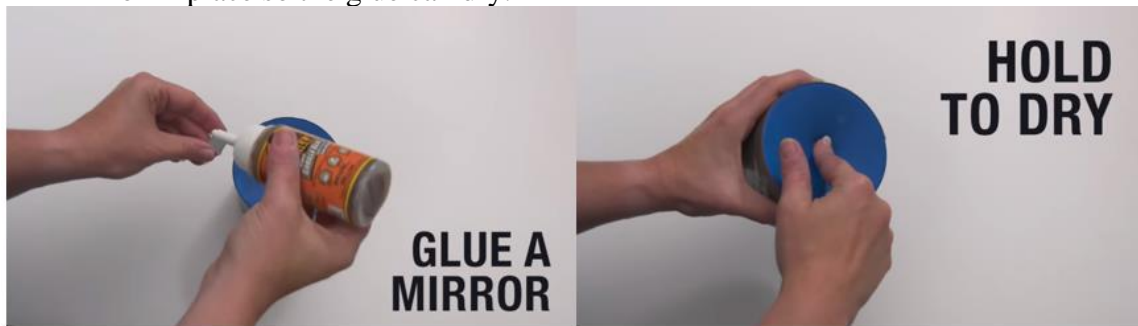
Figure 4. Glue the mirror to the center of the balloon
