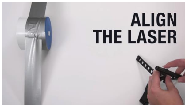
Figure 7. Align the laser so the light beam reflects off the mirror onto the wall
