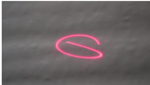
Figure 8. The light should move on the wall in response to the sound
