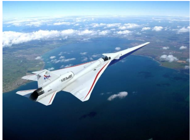
Figure 7. The X-59 (QueSST) is designed to fly supersonic without creating a sonic boom.
