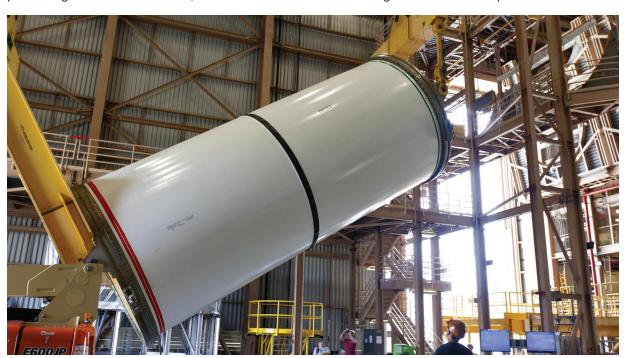
Technicians watch as a crane and special mechanism begin breakover, or flipping, of the mated Thrust Resistance Structure and Guidance Control Assembly for the Orion Program's Ascent Abort-2 flight test during practice, or pathfinder activities, June 22, 2018, inside the Rotation, Processing and Surge Facility at NASA's Kennedy Space Center in Florida. Photo credit: NASA/Ben Smegelsky
