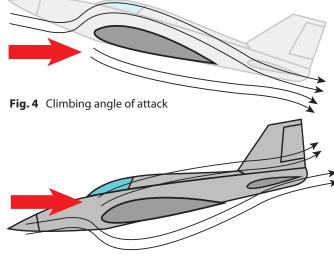
**Fig. 5** Descending angle of attack
