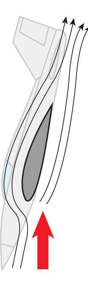
Fig. 5 Descending angle of attack
