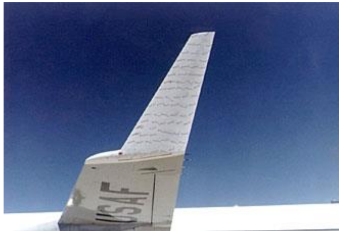
Figure 8. Winglets help reduce air vortices.
