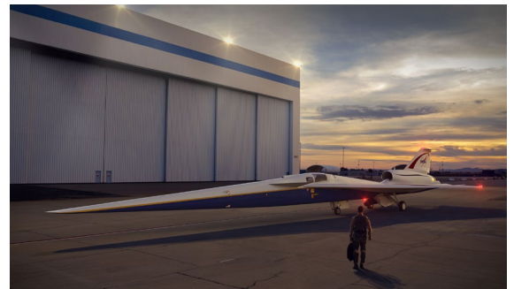
Figure 2. The X-59's unique design reduces the sonic boom to a quieter sonic thump.
